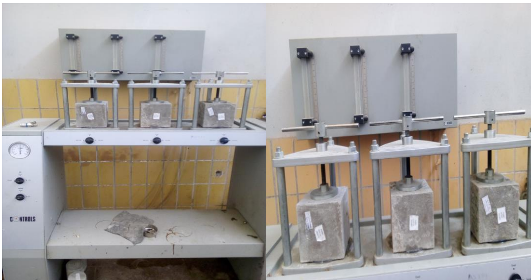
Figure 3-35: Machine and material setup for water penetration test
