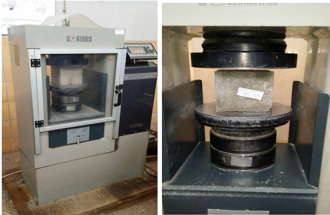
Figure 3-32: Machine and material setup for cubic compression test
