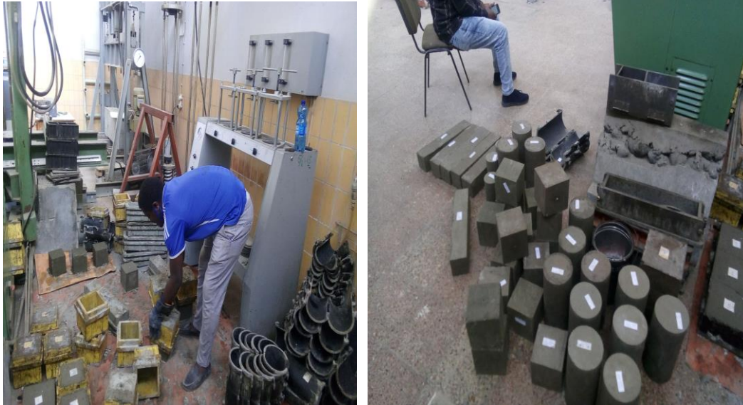
Figure 3-30: Concrete sample removed from the mold for curing
