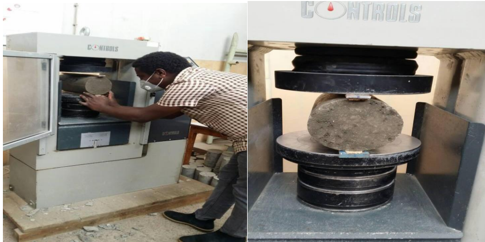
Figure 3-33: Testing set up for split tensile strength of concrete
