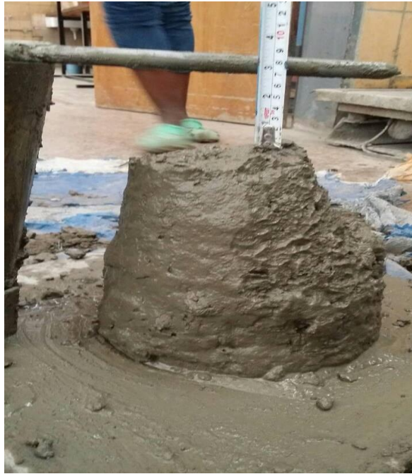
Figure 3-31: Slump test of the given concrete material
