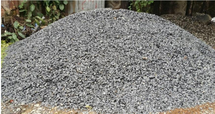
Figure 3-27: Coarse aggregate used for the concrete mix
