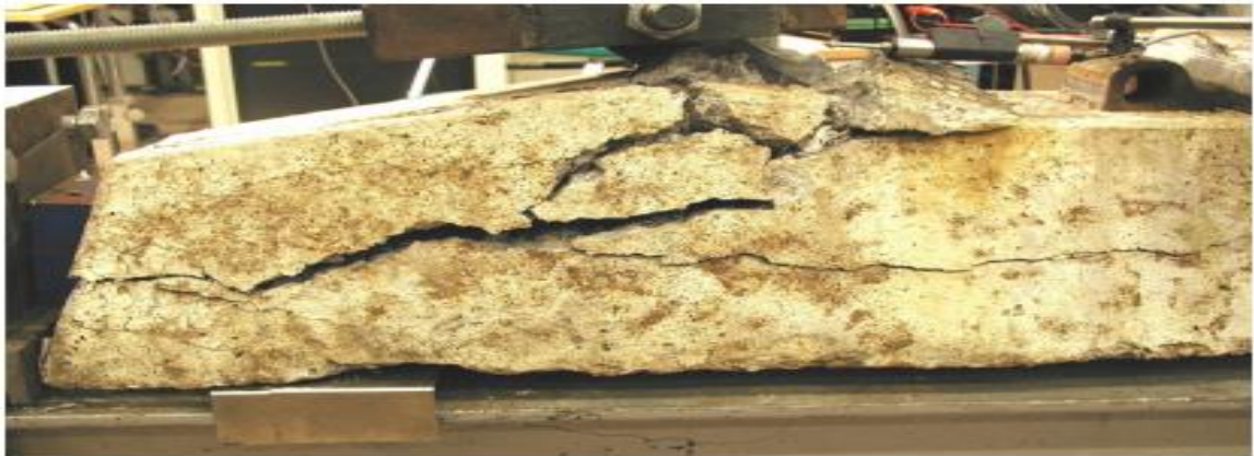
Figure 2. 5 Horizontal Cracking near the axle load
