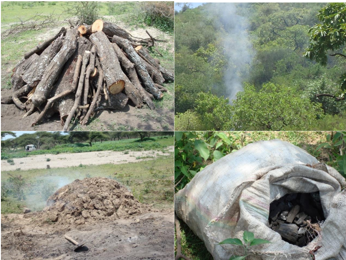
Figure 17 Traditional charcoal production using earth kiln
