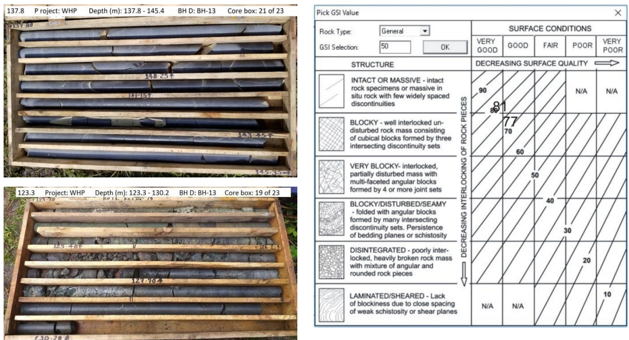
Fig. 5.4 GSI for BA-3 geotechnical unit. The drilled Core box shown on left is from BH-13 borehole and GSI value is shown on the right marked over standard chart proposed by Rock Lab Guide by Hoek and Brown, 2002.
