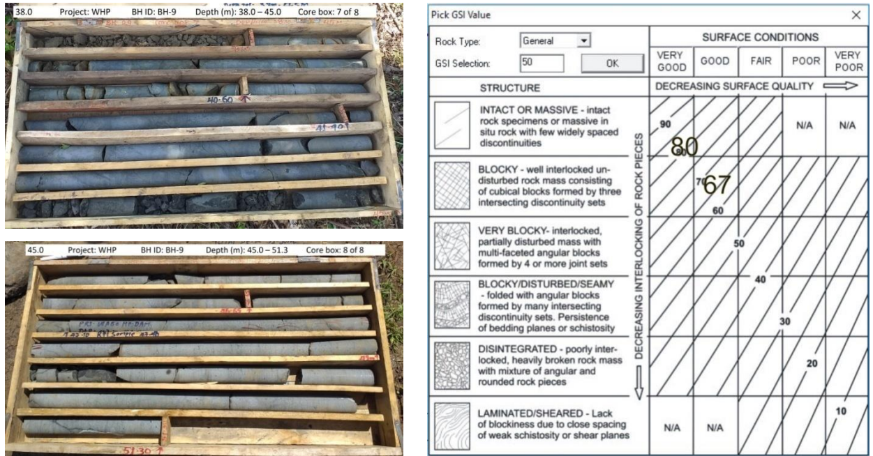
Fig.5.3 GSI for BA-4 geotechnical unit. The drilled Core box shown on left is from BH-9 borehole and GSI value is shown on the right marked over standard chart proposed by Rock Lab Guide by Hoek and Brown, 2002.
