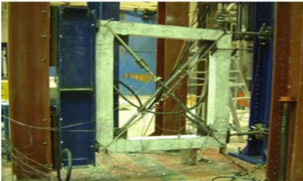
Figure; 2.2 Setup for cyclic testing of internal brace specimens
