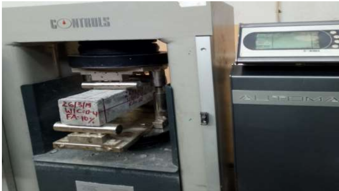
Figure 4-2: Sample set up for flexural strength test
