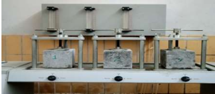
Figure 4-3: Water penetration test
