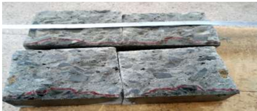
Figure 4-4: concrete sample just after splitting
