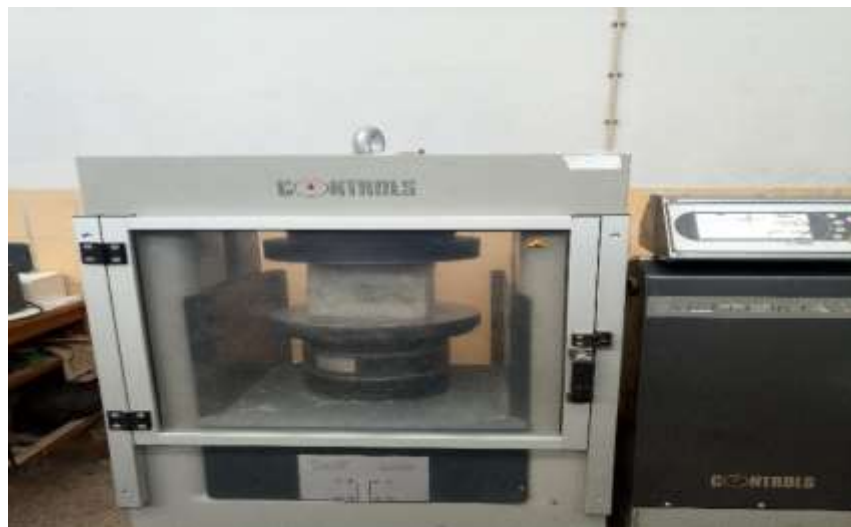
Figure 4-1: Sample set up for compressive strength test
