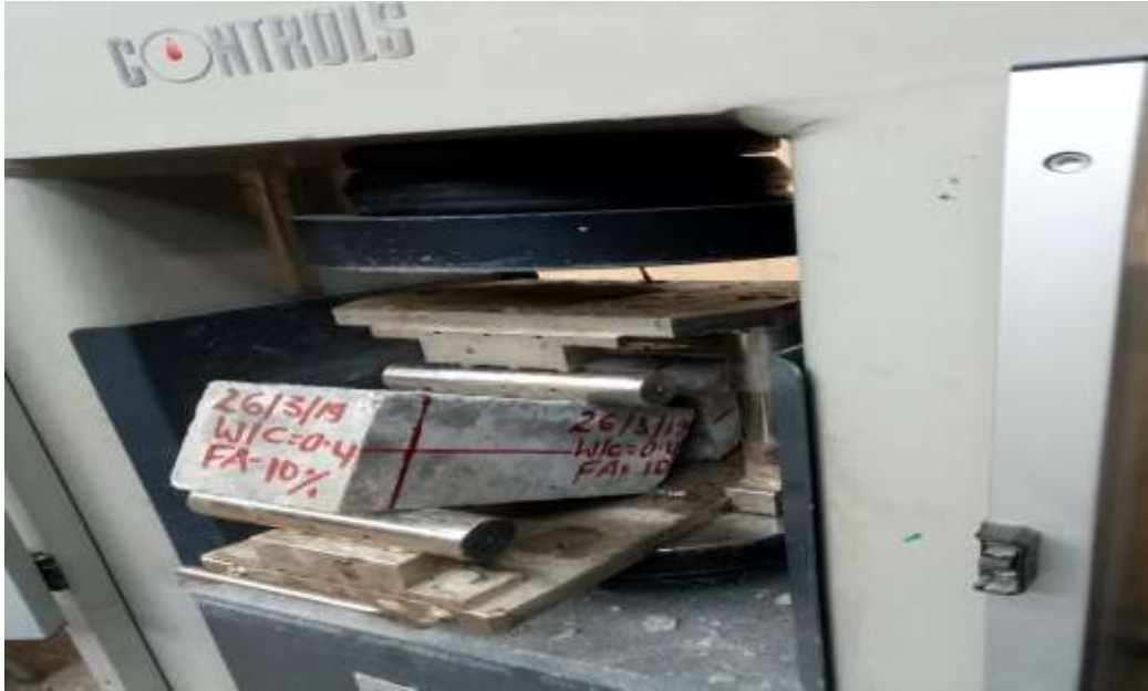
Figure 5-5: Beam failure during flexure test
