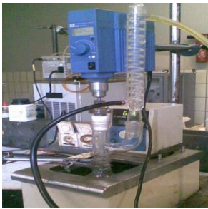
Figure 3.5 Experimental set-up for batch transesterification reaction
