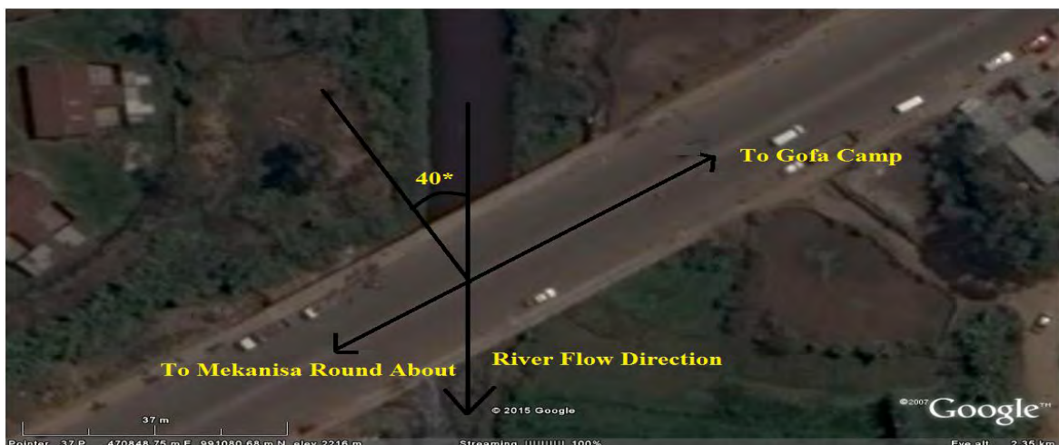
Figure 10. Angle of Skewness at Mekanisa Bridge
