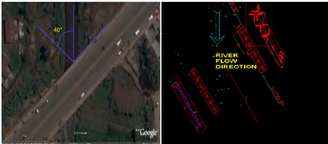
Figure 50. Skew angle and Bridge alignment with respect to the flow direction.
