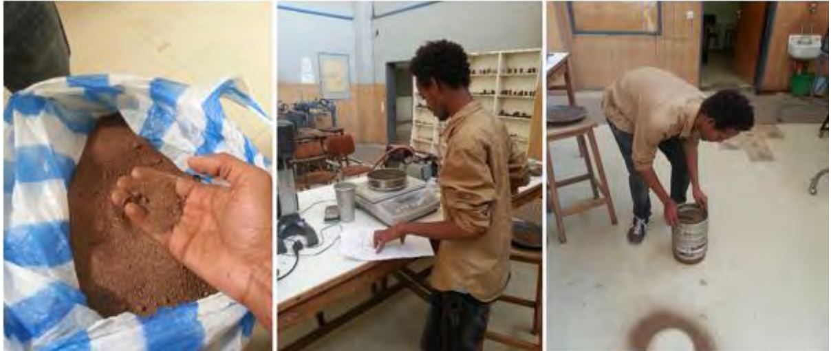
Figure 23. Soil sample and sieve analysis
