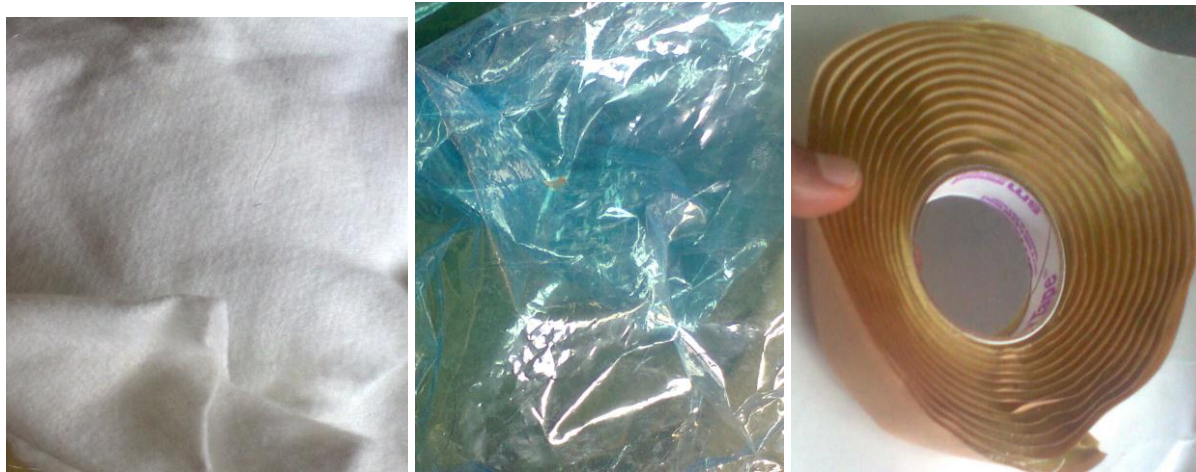
Figure 3.6: Materials used for vacuum bagging (a) Pressure Fabric or Breather (b) Vacuum nylon or Vacuum Bag (c) Mastic sealant (Vacuum tape)
