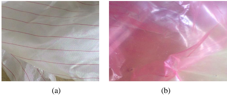
Figure 3.5: Materials used for vacuum bagging system (a) released fabric (peel ply) (b) Perforated nylon
