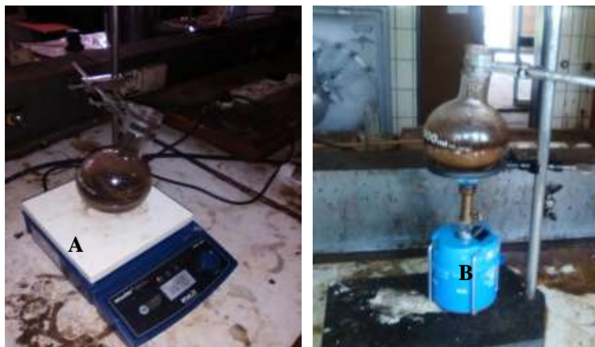
Figure 3. 12 Digestion stage: (A) for GM and (B) for MFW
