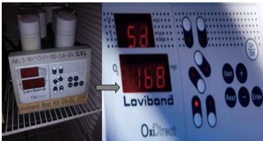
Figure 3. 10 Lovibond® OxiDirect BOD measuring system incubated with samples
