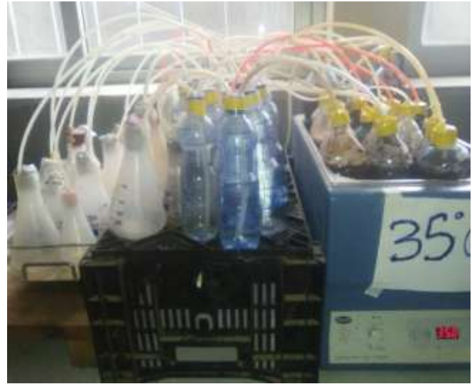
Layout of the experimental setup at operating Temperature of 35° C
