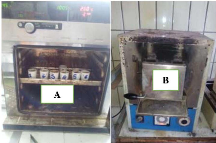
Figure 3. 5 TS and VS determination: drying oven (A) and muffle furnace (B)
