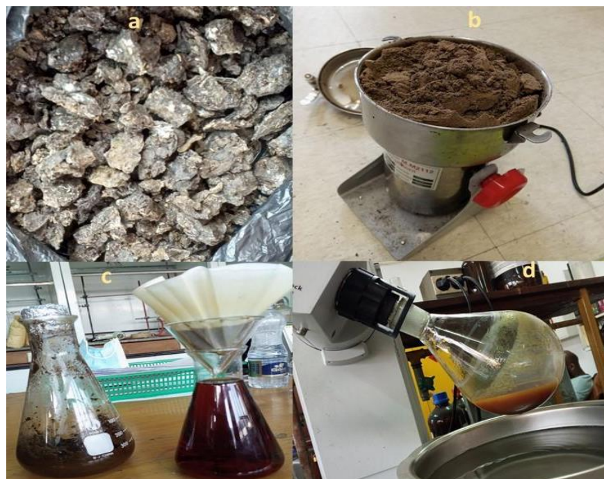
Figure 6. 1 Extraction process of crude propolis collected from honeybee colonies a) Crude propolis b) Grinded propolis c) Filtration of extracted propolis d) Concentrating using rotary evaporator
