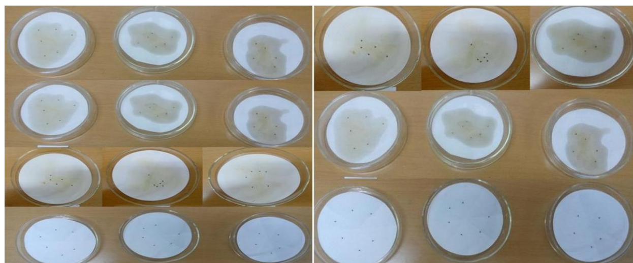
Figure 6. 2. Different concentration bioassay test of propolis extracts on V. destructor mite
