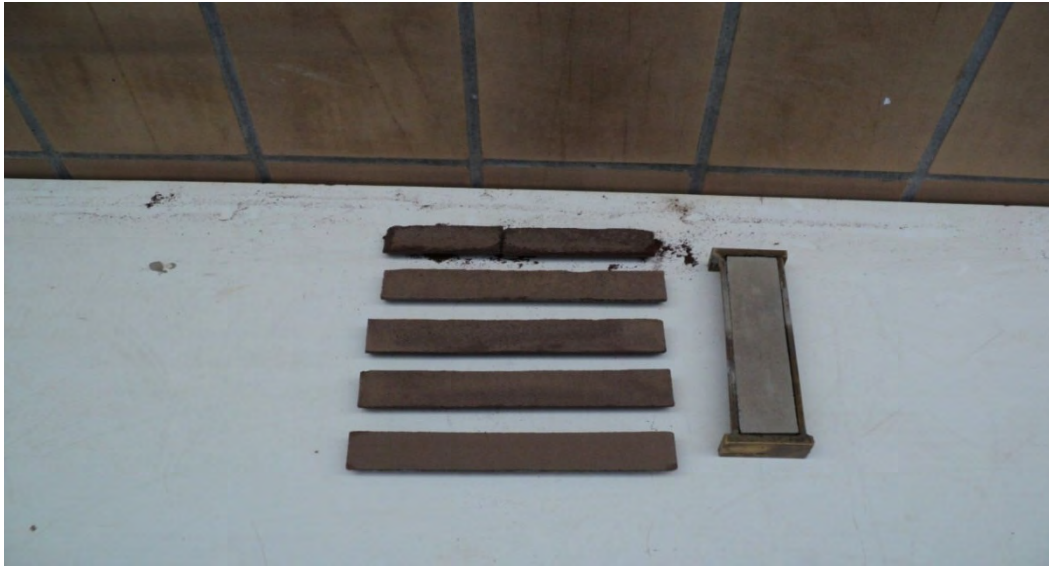
Figure 4.14: Oven-dried specimen for different proportion of fine-grained soil
