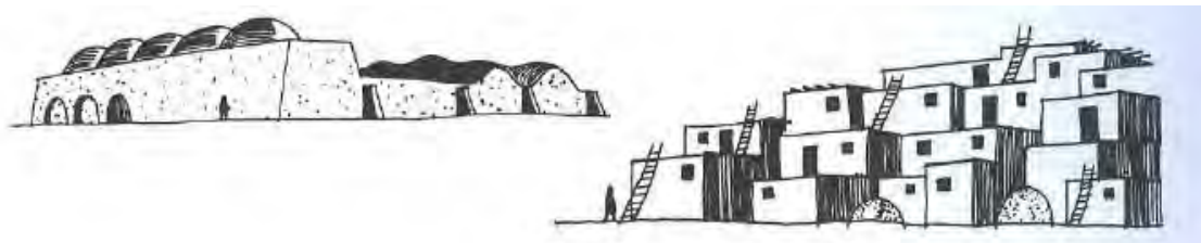
Fig. 3:6 Dwellings made of one material (mud). Left: Iran. Right: Pueblos, south western United State
