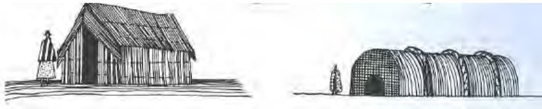
Fig. 3:5 Dwellings made of one material (reeds). Left: Uru dwelling, Lake Titicaca, Peru. Right: Marsh Arab dwelling, Iraq-Iran border Source Rapoport (1969)
