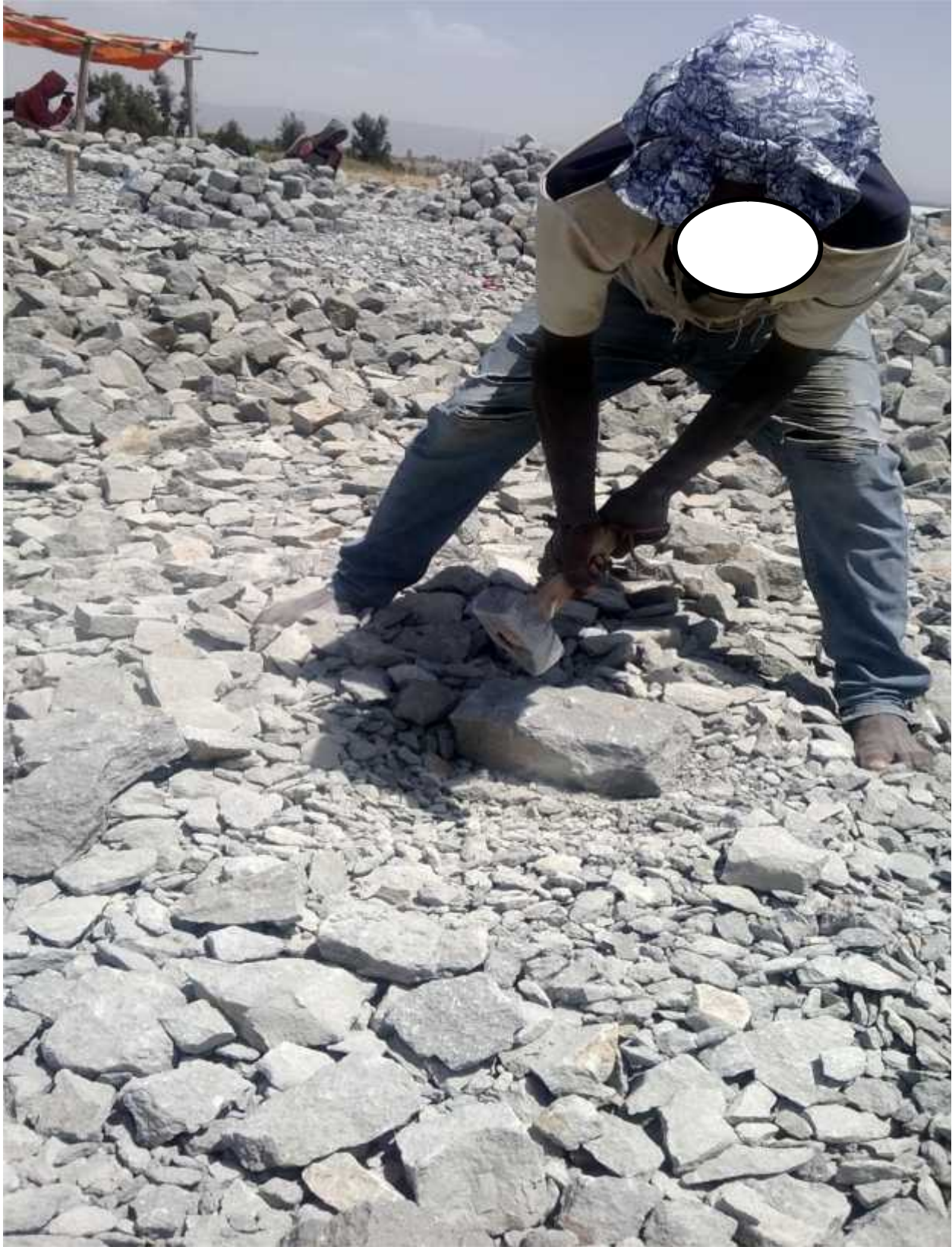
Figure 6: photos of chiseling activity at cobblestone sites in Addis Ababa
