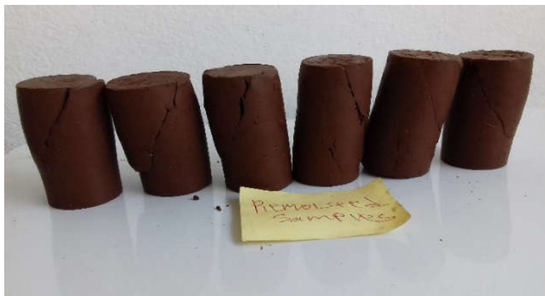
Figure 5-7 summary of failure pattern for remolded samples at the rate of (0.37 to 1.75) mm/min
