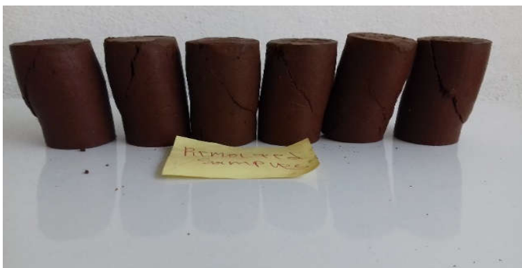
Figure 5-9 summary of failure pattern for remolded samples at the rate of (0.23 to 1.14) mm/min
