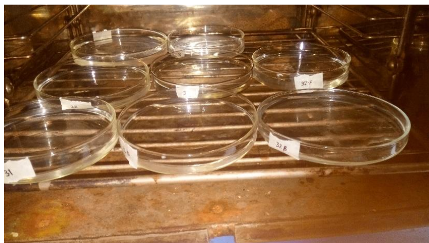
Figure D-2 Crosslinking reaction of Polymer solution inside the oven
