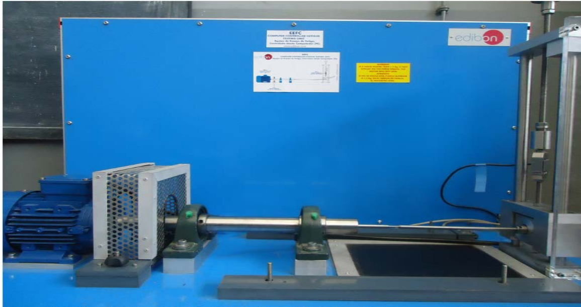
Figure 3.15: Specimen placed in the fatigue testing unit machine
