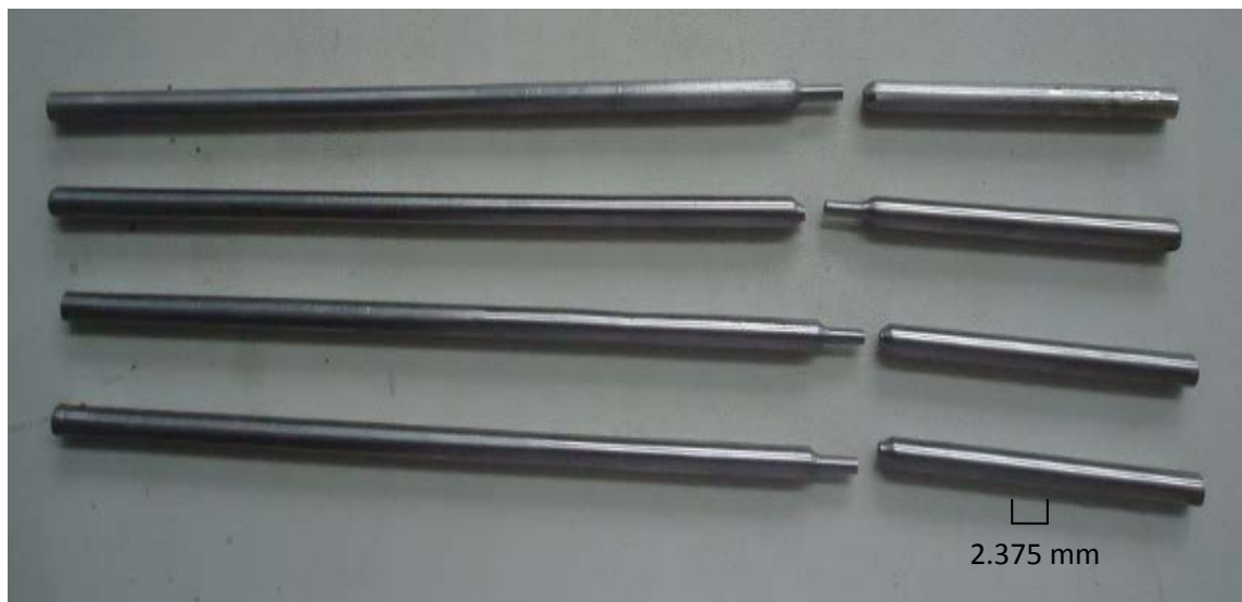
Figure 4.16: Specimens failed on fatigue test
