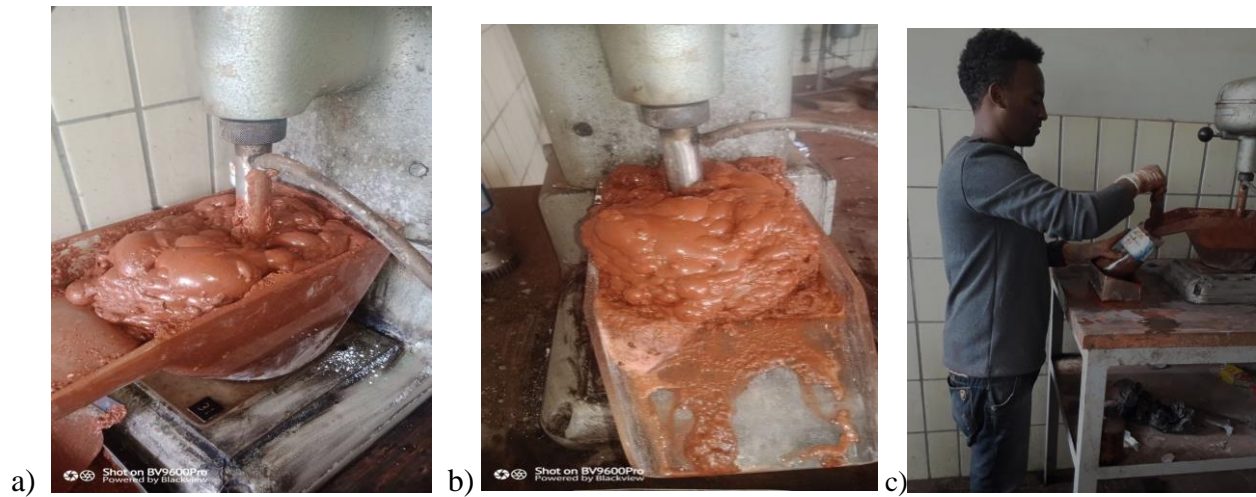
Figure 8: a, b and c show flotation of hematite ore and.
