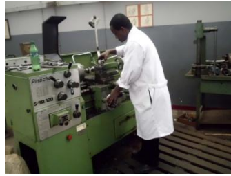
Figure 11 the raw alloys go through machining process on a lathe machine.
