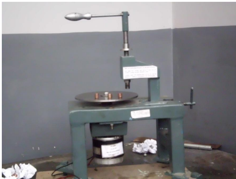
Figure 14 the pin-on-disk tribometer for the wear test, and some sample alloys.
