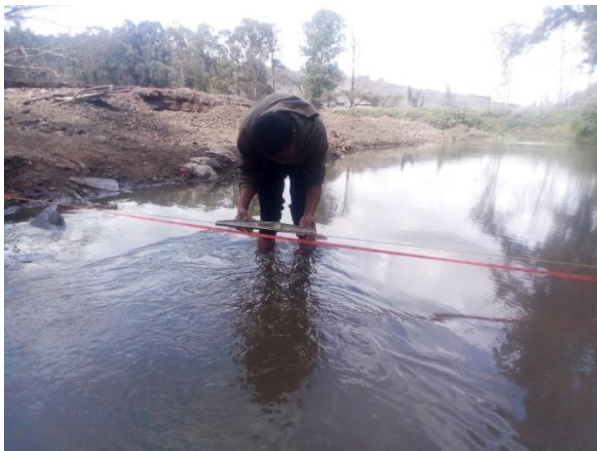
e. Establishing the difference in elevation b/n the stakes
