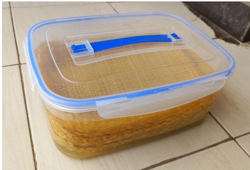
Figure 14 The fiber treatment (with 2% NaOH solution for 4hrs)
