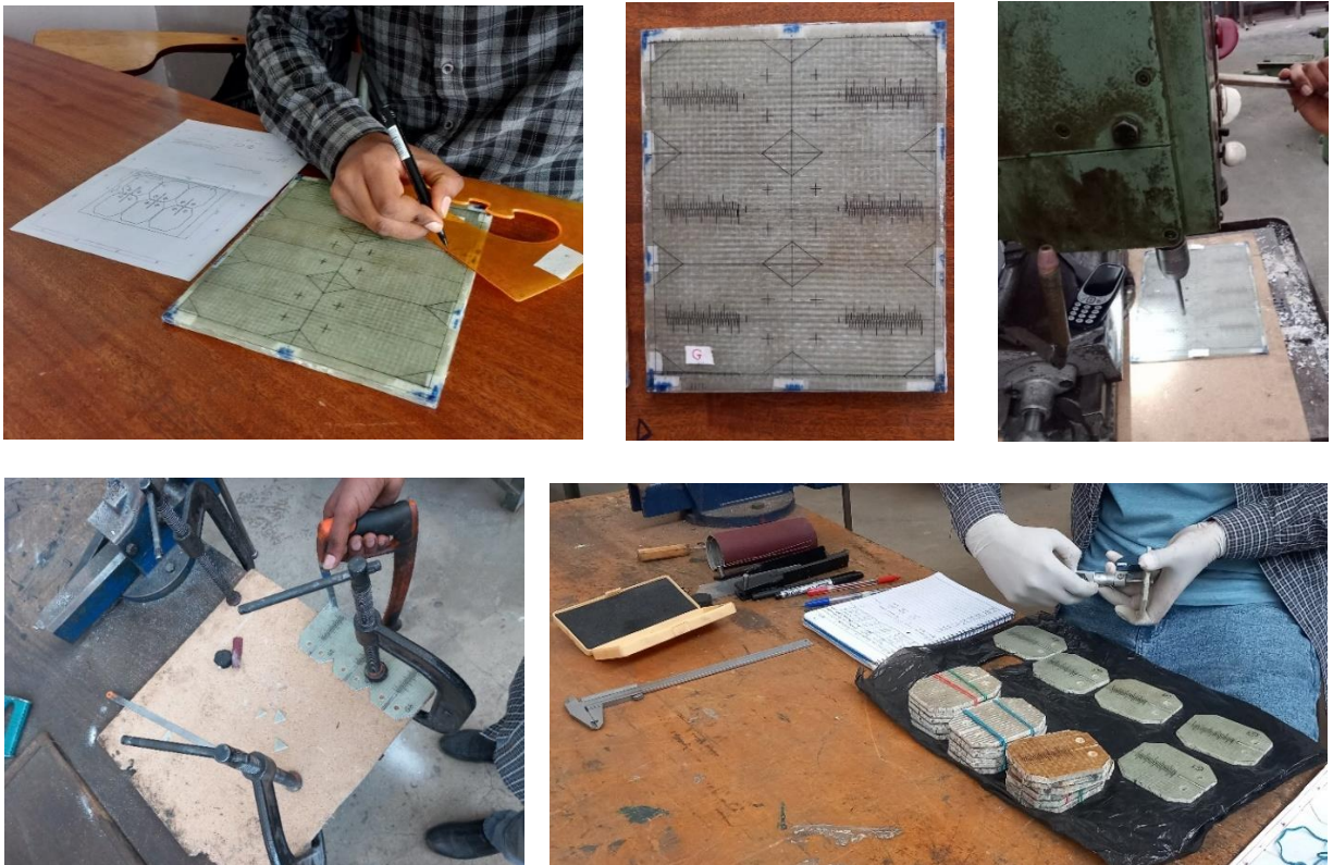
Figure 21 Specimen marking, drilling, cutting and measuring process
