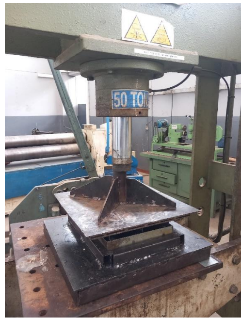
Figure 18 The hand layup and compression molding process
