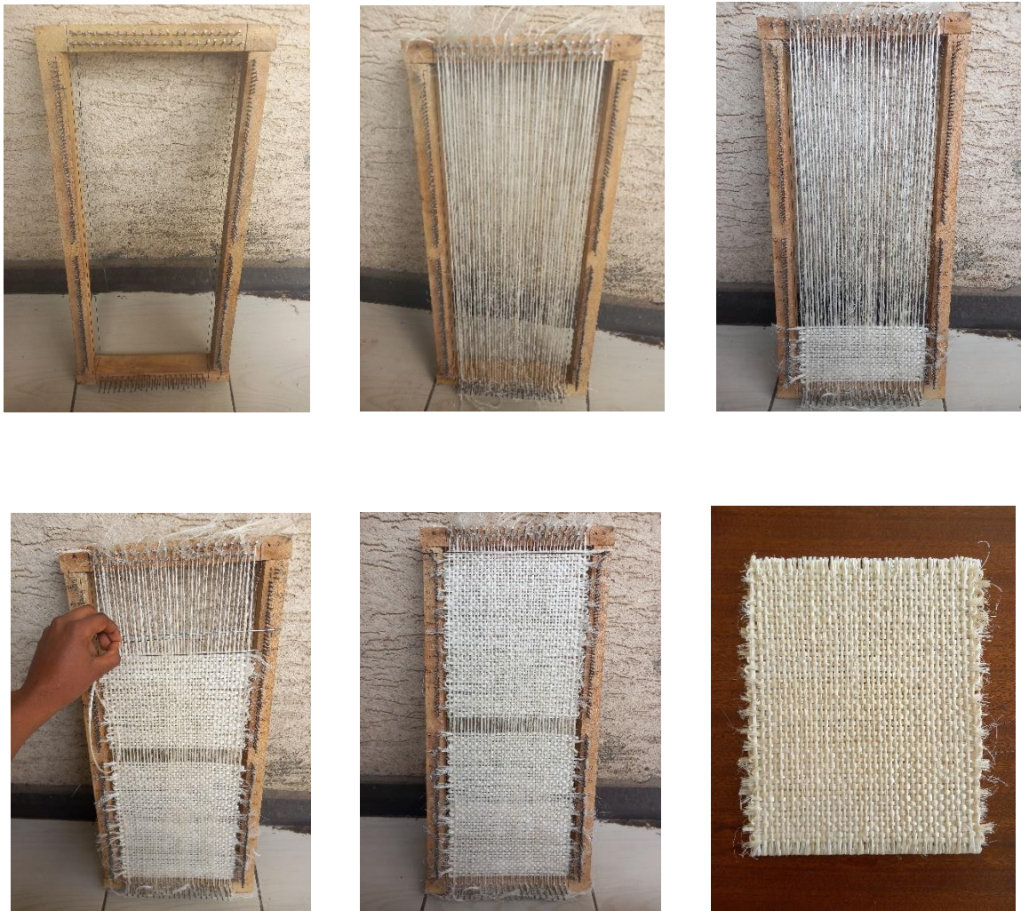
Figure 13 The hand weaving process
