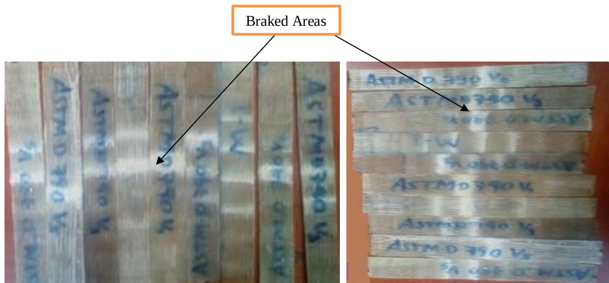
Figure 4-7 Failure mode of ENF specimens
