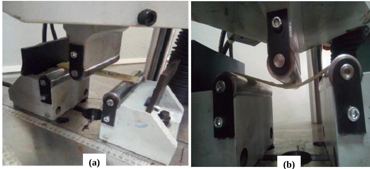
Figure 3-16 ENF Test setup on WAW 600D UTM, (a) before operation takes place (b) in loading Based on the experimental data, the mode II fracture resistance can be evaluated by using the following equation:
