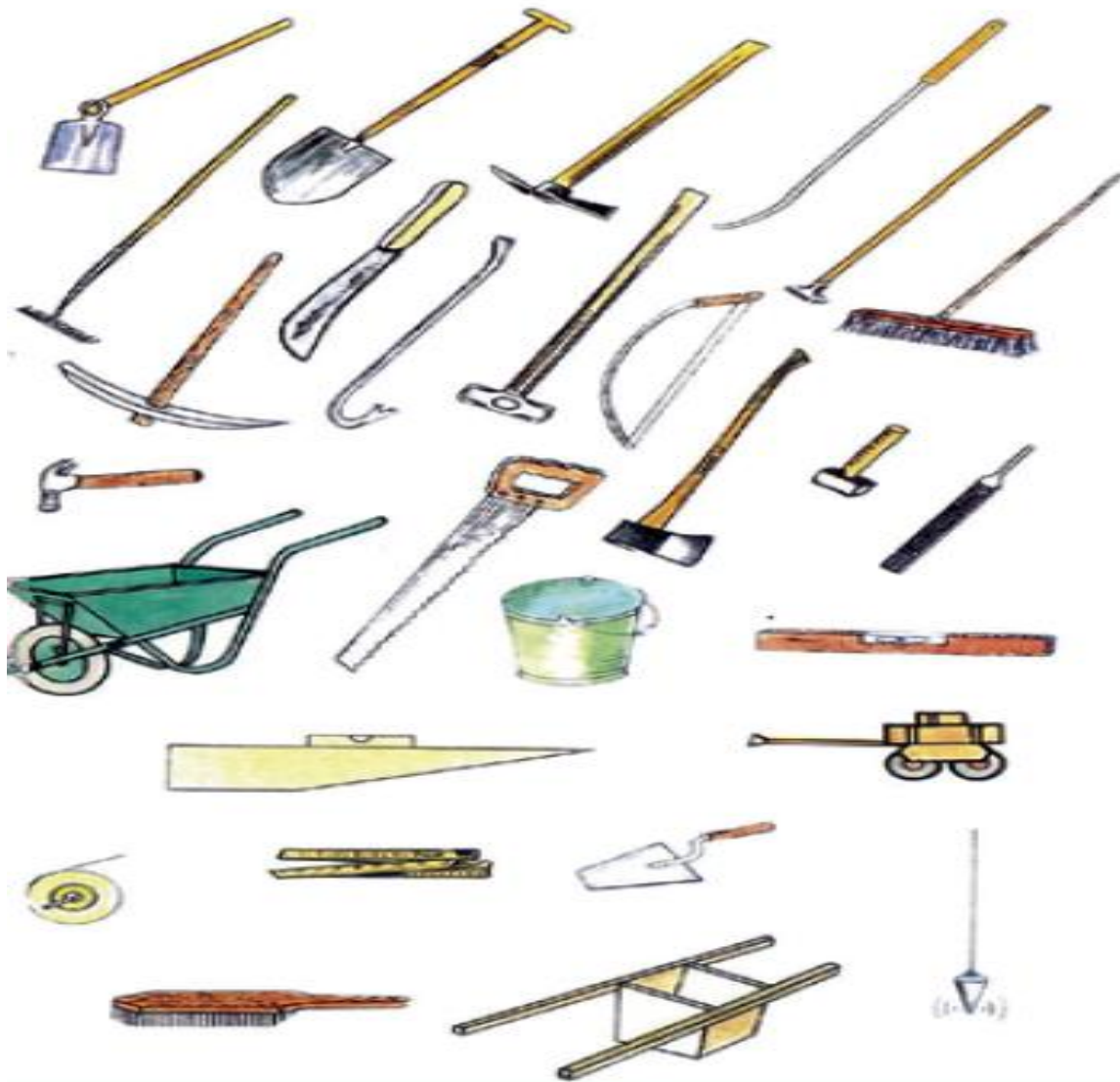
Figure 5.2: Range of Simple Tools and Control Aids sound for URRAP Roads' Maintenance (Source: ERA, 2011)
