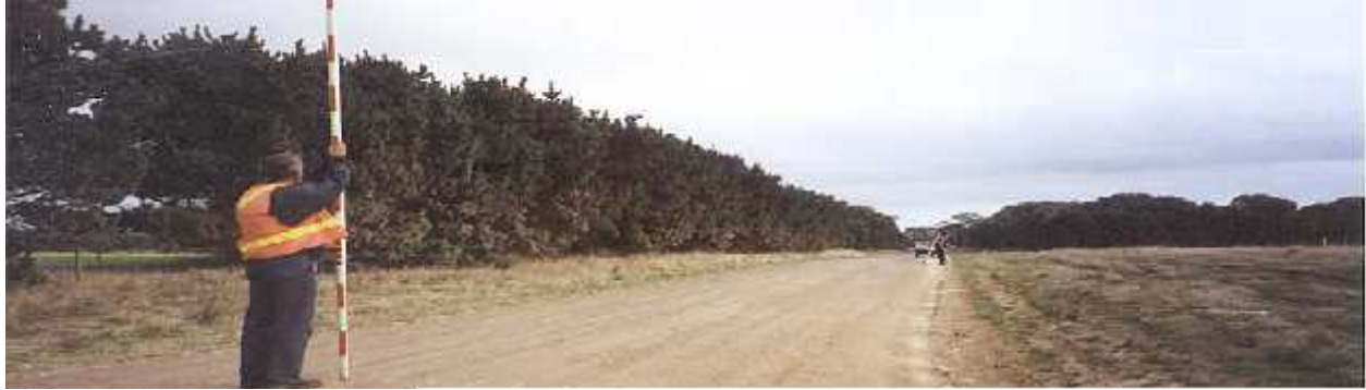
Figure 2.20: Measuring gravel loss on the field
