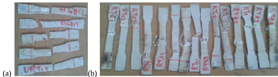
Fig. 4.9 Comparison of the strength of URP and RP under Uni-axial loading
