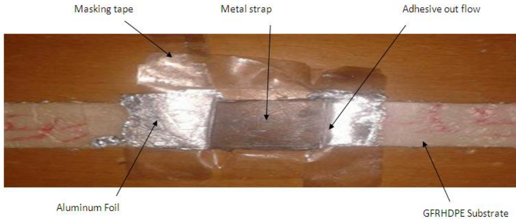
Fig. 3.2 The adhesively bonded single strap joint
