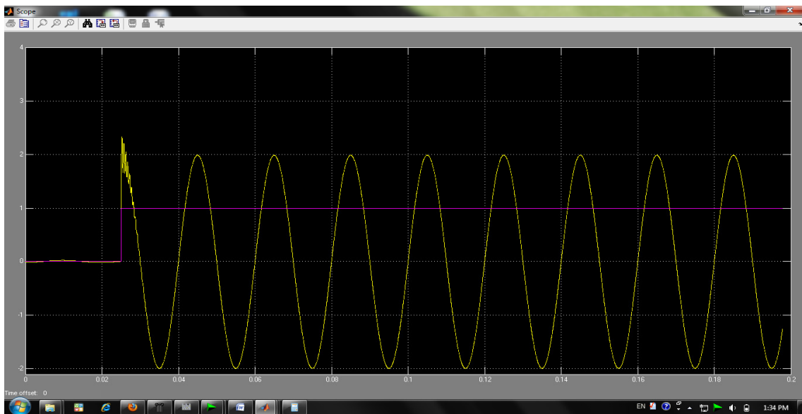
Figure 5.2 Simulation result of transient reduction using 5-unit compensator.
