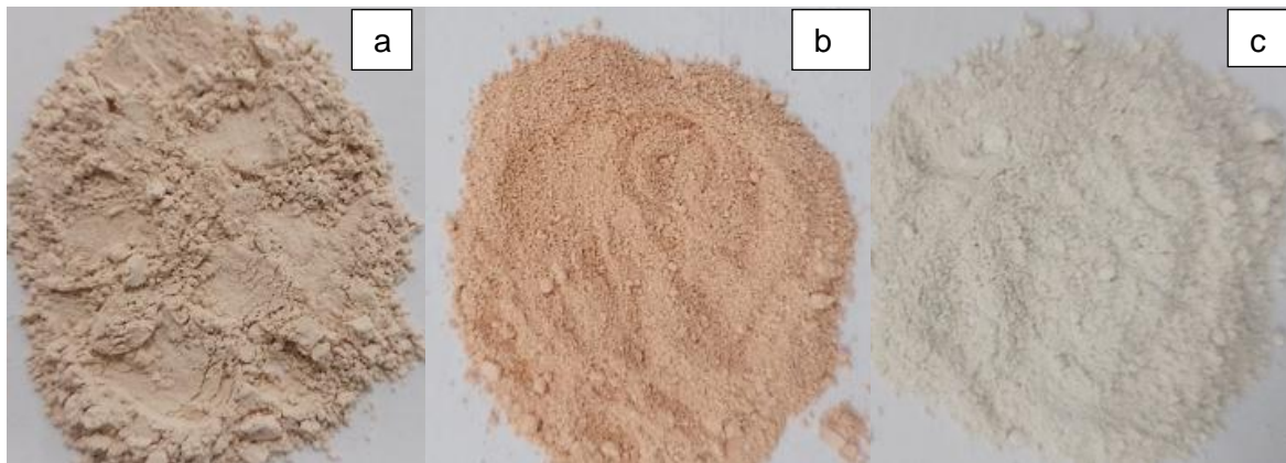
Figure 16. Powder Samples of (a) raw kaolin ;(b) wet beneficiated and calcined kaolin; (d) wet beneficiated and acid leached.
