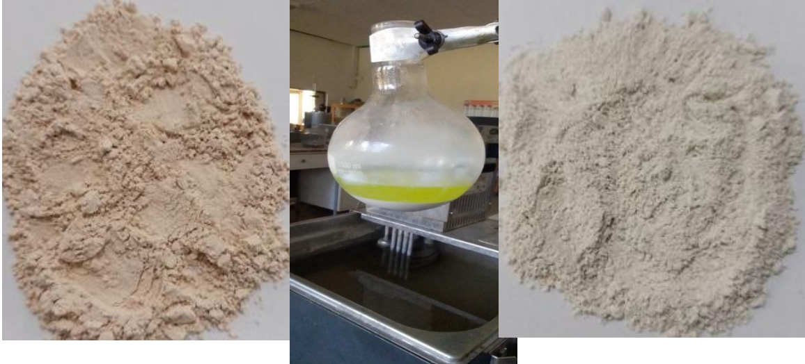
Figure 15. Chemically bleached kaolin's intended for high-value applications.
