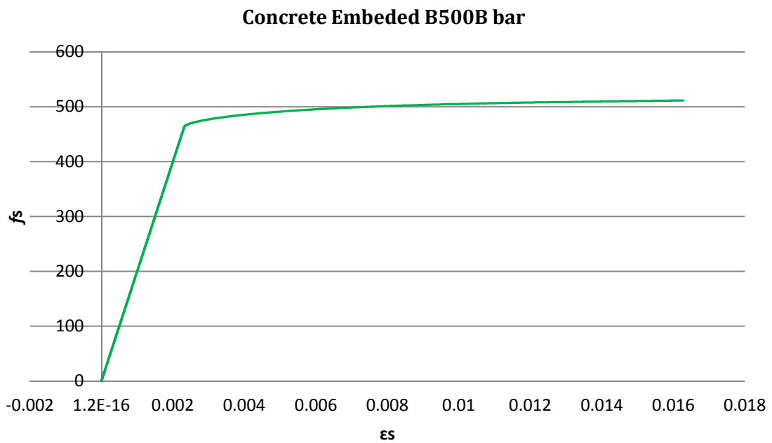
Figure 3-9: Stress vs. strain diagram of bare reinforcing bar under tension
