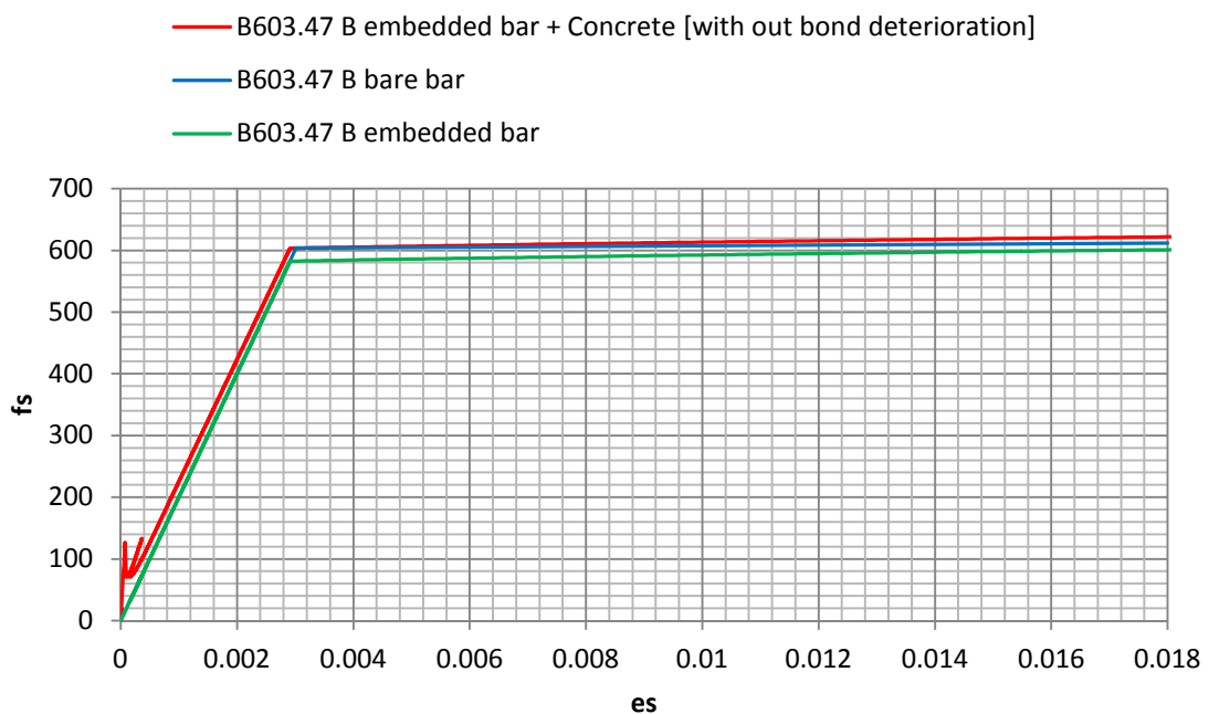
Figure 4-6: Comparison of the three stress vs. strain diagram in tension for the proposed effective concrete section in the tension zone designated as proposed approach max.
