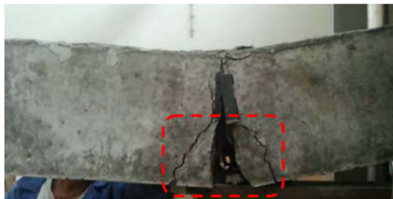
Figure 2-5: Splitting conical cracks
