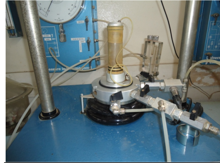
Figure B-3: mounted soil sample on triaxial machine.
