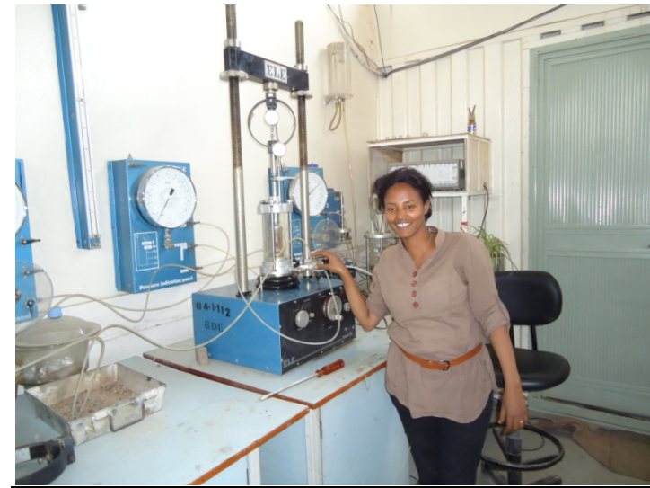
Figure B-4: conducting isotropic consolidation triaxial compression test.
