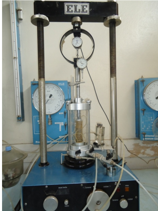
Figure 3.8: Triaxial compression machine.
