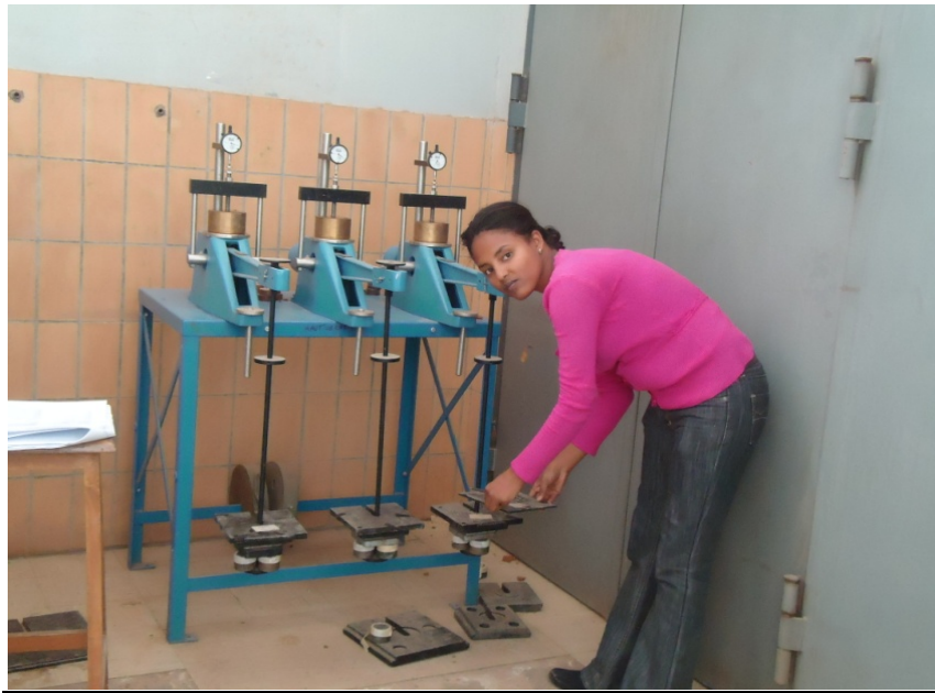
Figure B-2: Loading one dimensional consolidation machine.
