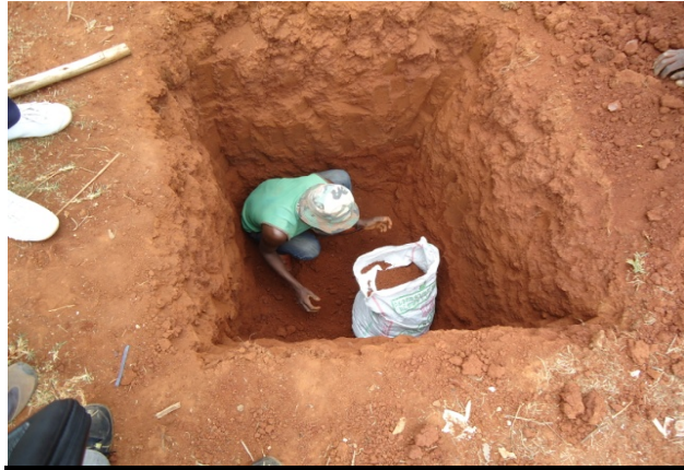
Figure B-1: Extracting disturbed soil sample.
