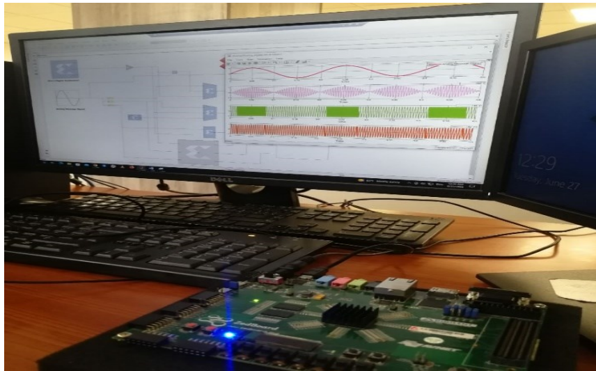
Figure 5.5 (a): Analog Modulation system result after Implementation
