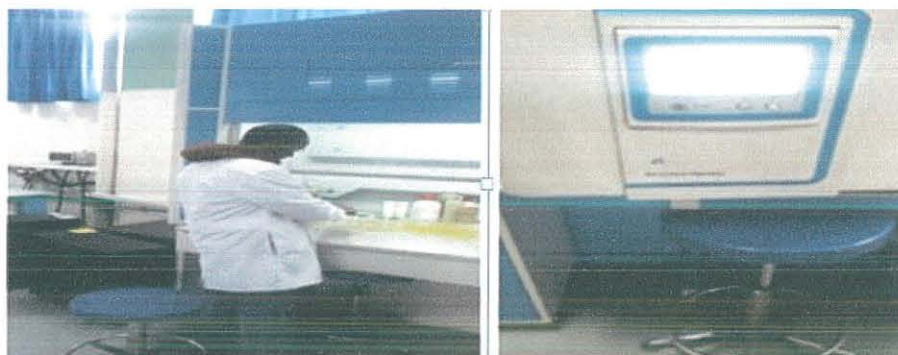
Figure 6: Microwave digestion of vegetable samples for mineral analysis
