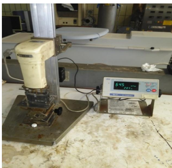
Figure 0.2B Indicates viscosity value- with viscometer
