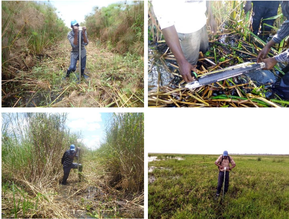
Figure 3.1 Taking soil samples in the natural and rice paddy sections of the wetland
