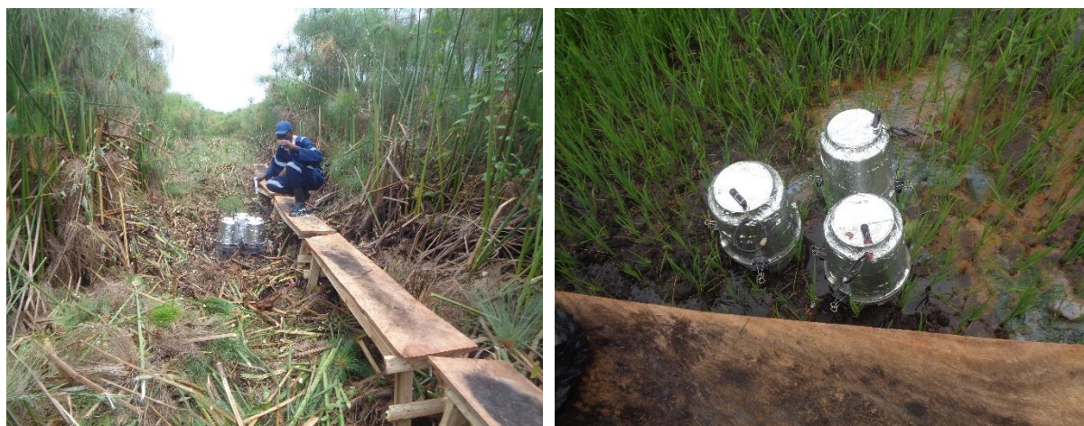
Figure 5.1 Taking gas samples in the natural (Left) and rice paddy (Right) sections of the wetland
