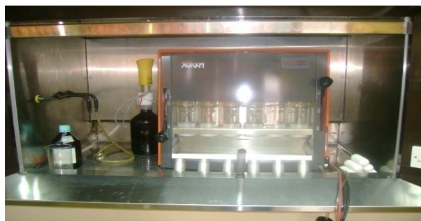
Fig 3.4 Crude fat extraction unit
