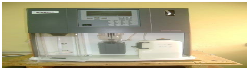
Fig.3.3 Protein analyzer unit
