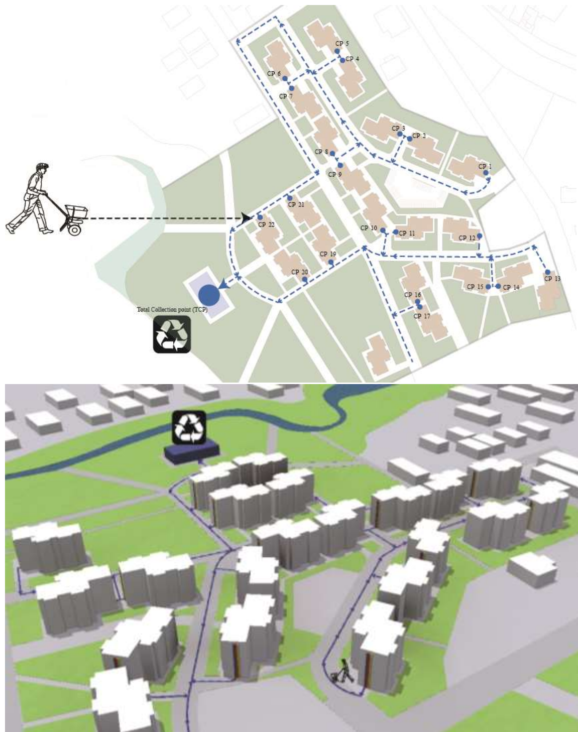
Fig 5.2: Proposed movement for organic solid waste collection point for “Basha Wolde-Chilot” condominium
