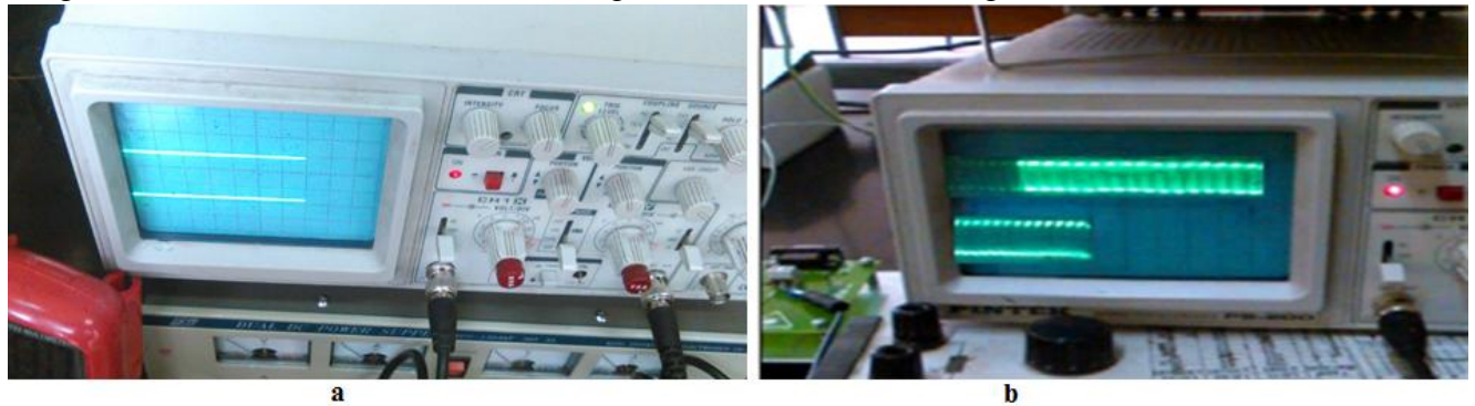
Figure 48 Oscilloscope (a) dual channel zero reading (b) reading after input and output were connected.
