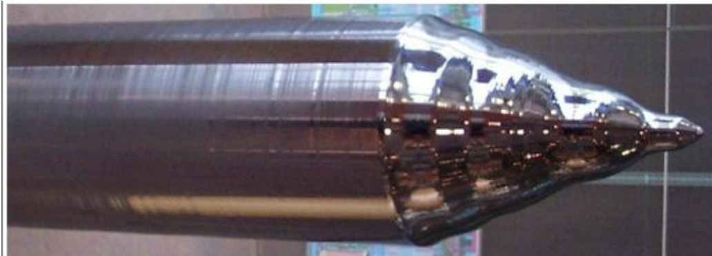
Figure 33 Crystal of Czochralski grown silicon [40].
