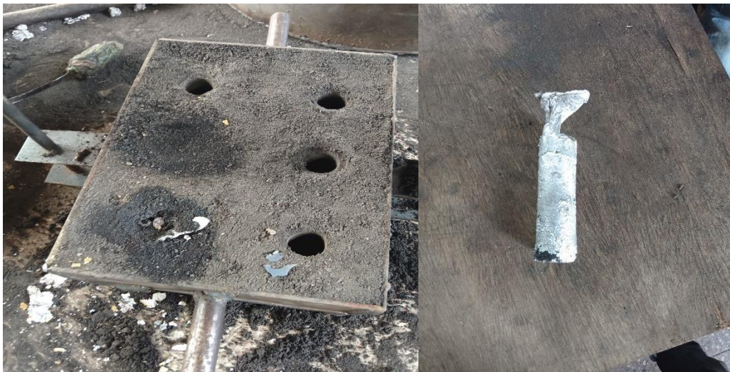
Figure 3.7. Molten metal poured in the sand mold and the cooled composite specimen.
