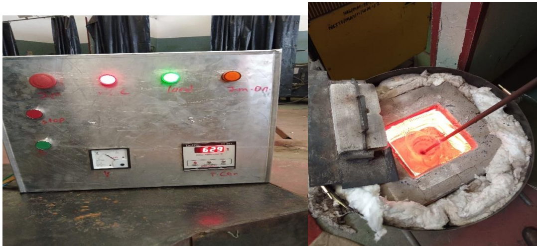
Figure 3.4. Molten composite material in the furnace at 629°C.
