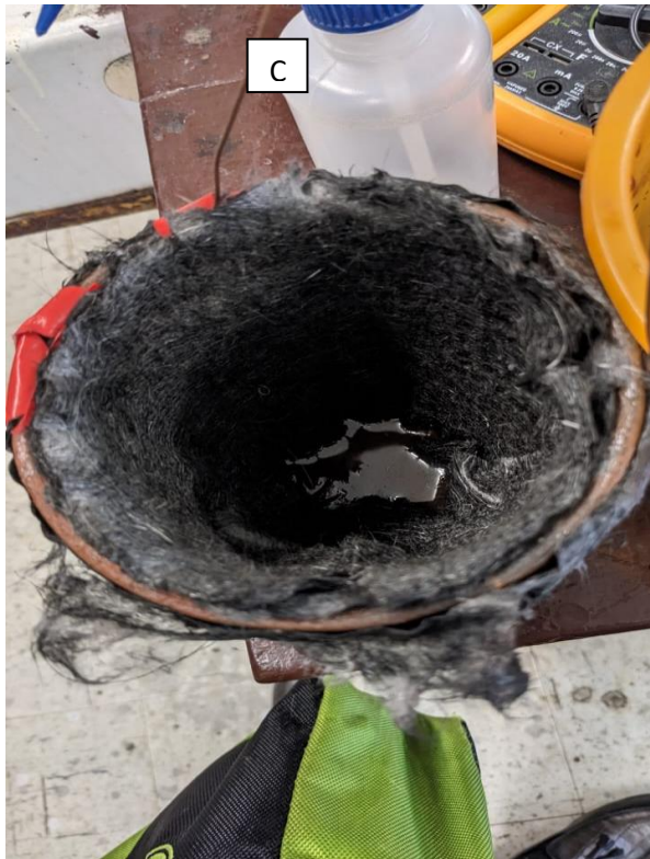
Figure 9 .Biofilm formation on the anode for A: MFC1, B: MFC 2 and C: MFC control
