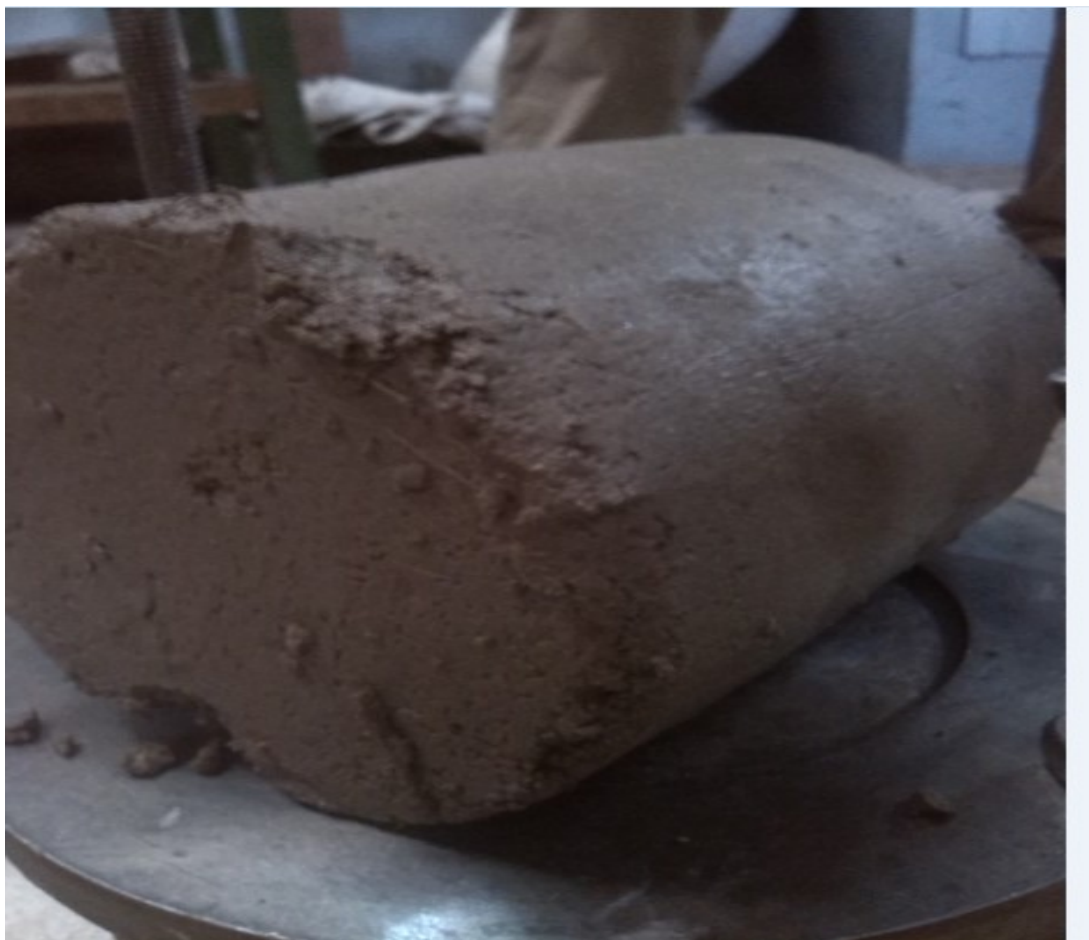
Figure 4.3: Reinforced soil with bamboo after compaction (High ductility)
