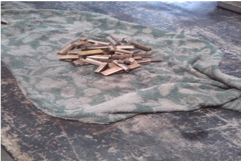
Figure 4.11: Water absorption test on bamboo (Removing of excess water)
