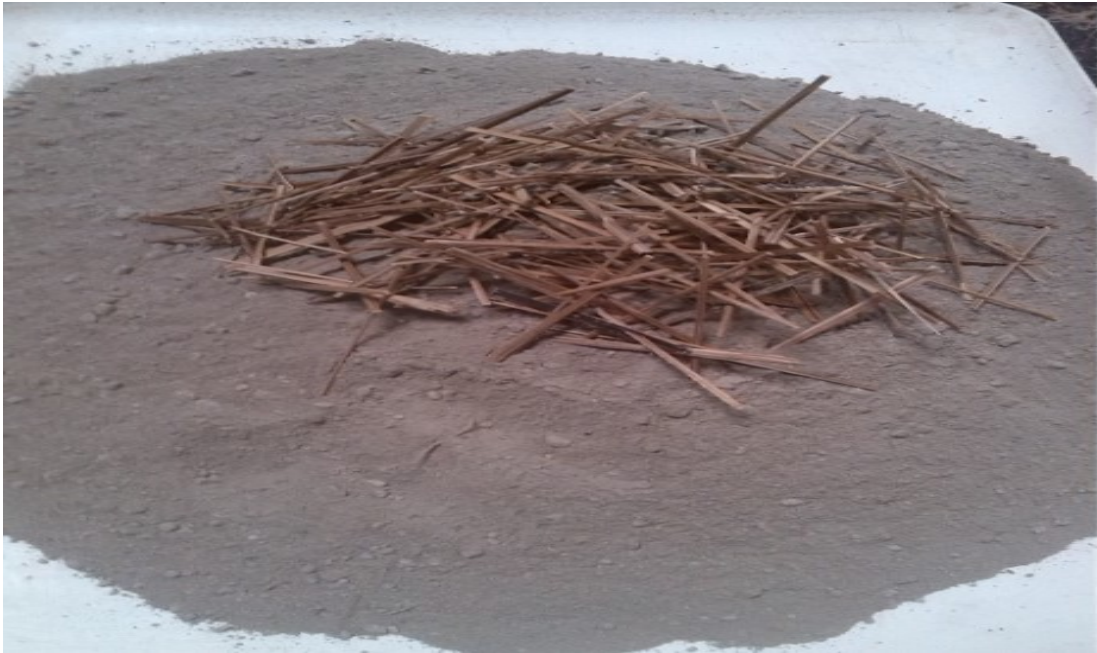
Figure 4.2: Preparation of sample for compaction (Reinforced soil)
