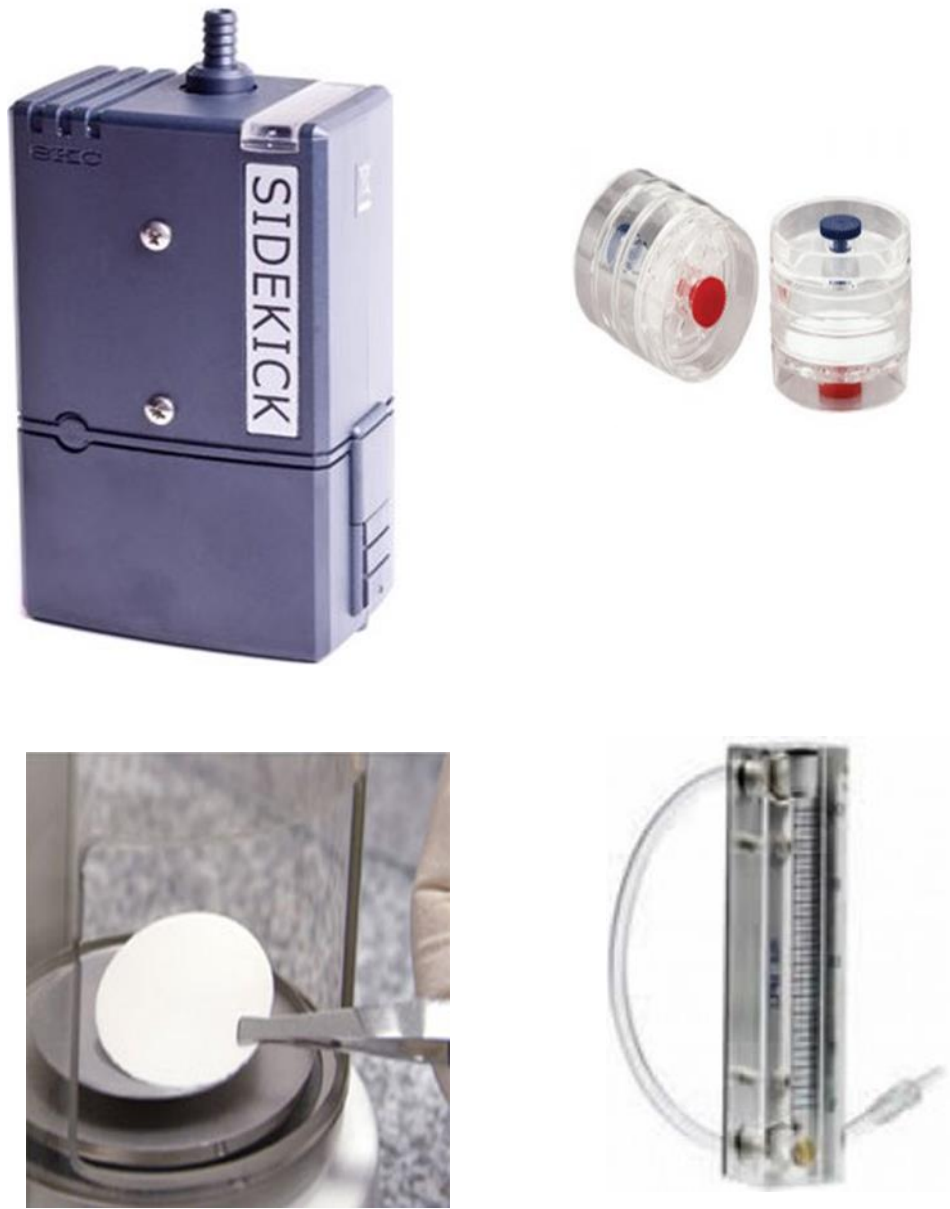
Figure 9: Dust sampling equipments used among street sweepers in Addis Ababa, Ethiopia, 2018, i.e., Hand pump, 37 mm Millipore plastic cassette (CFC), PVC filter, and Rota meter respectively.
