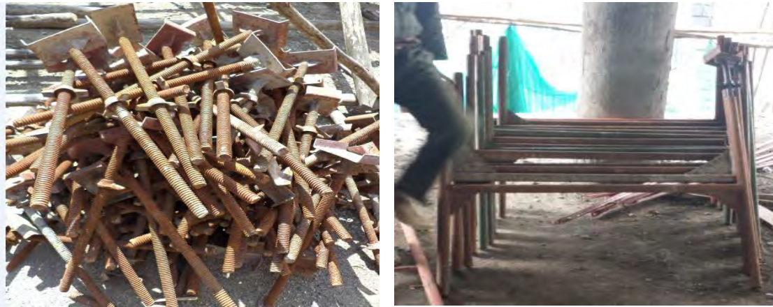
Figure 4.3 Adjustable u-head, Base plates and mini frames
