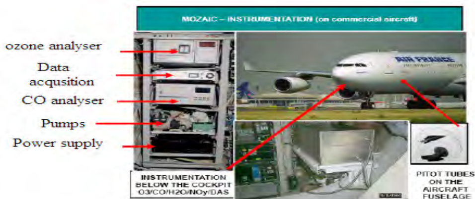
Figure 4.2: View of the removable plate with probes: Pitot tube ( O_3 ) sampling and Rosemount housing ( H_2O and temperature sensors), installed on a MOZAIC A340 airbus.
