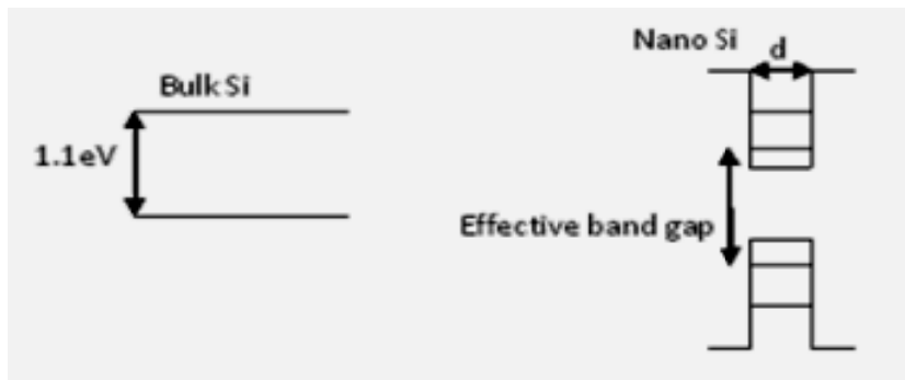
Figure 3 Energy band gap of the bulk Si system and that in the typical nanocluster. The presence of singularities in the DOS is easily discernable from the band electronic structure of the nanocluster [12].
