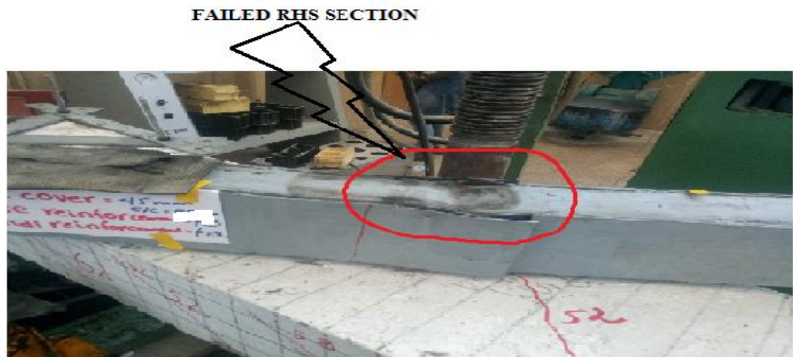
Figure 4-13 Failed RHS section during taking test NSC_S2_C30
