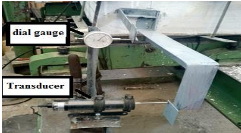
Figure 3-15 Angle of twist measurement using transducer and dial gauge
