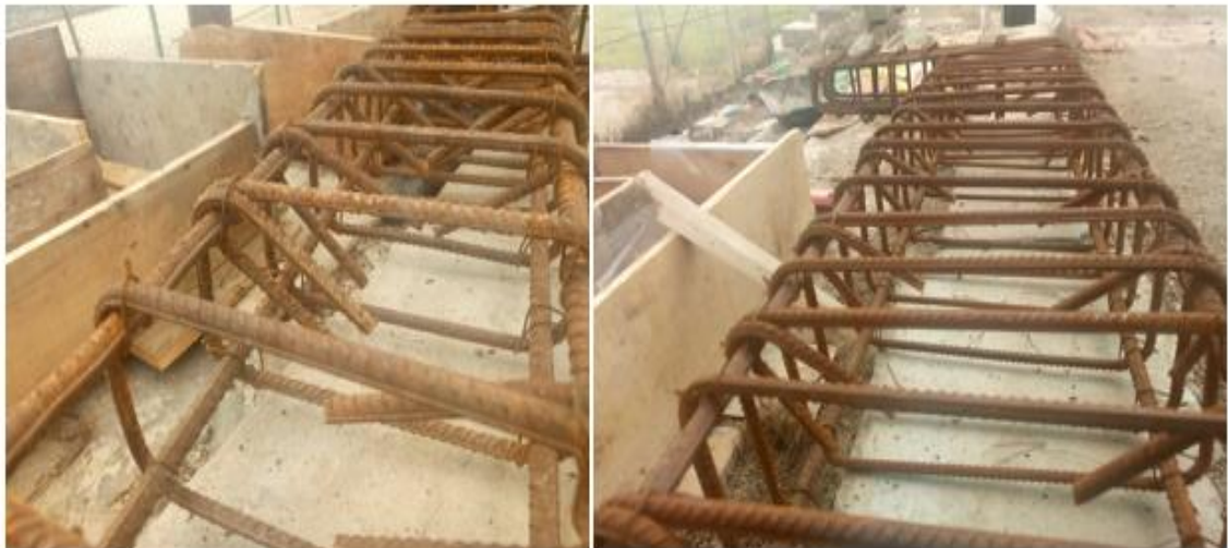
Figure 3-8 Specimen reinforcement preparation
