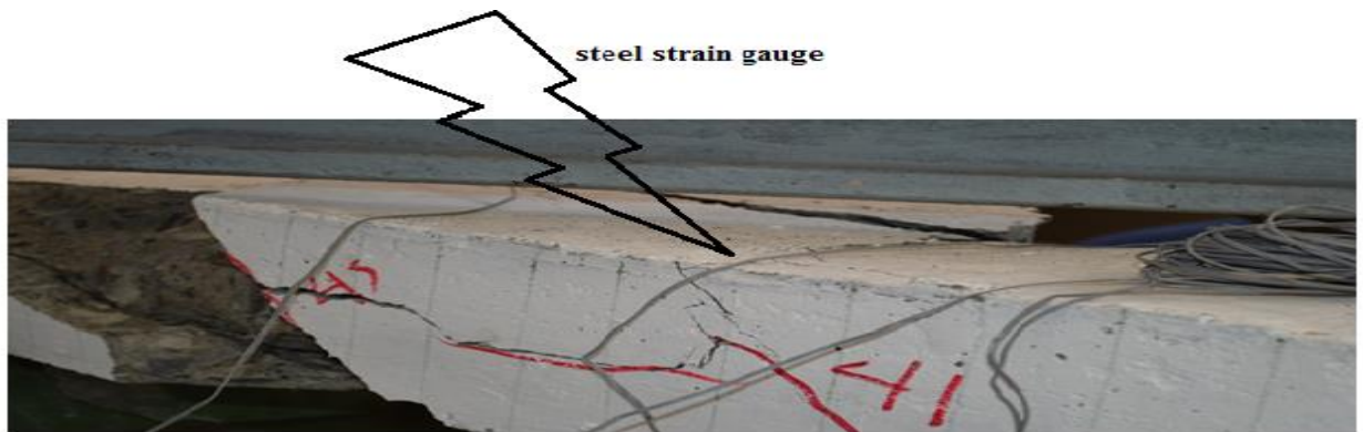
Figure 4-10 Attached steel strain gauge
