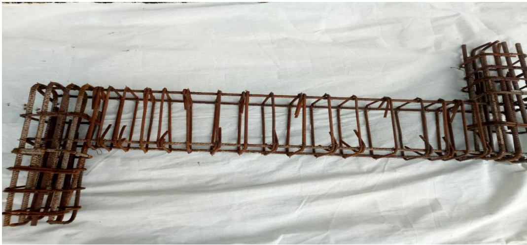
Figure 3-8 Specimen reinforcement preparation
