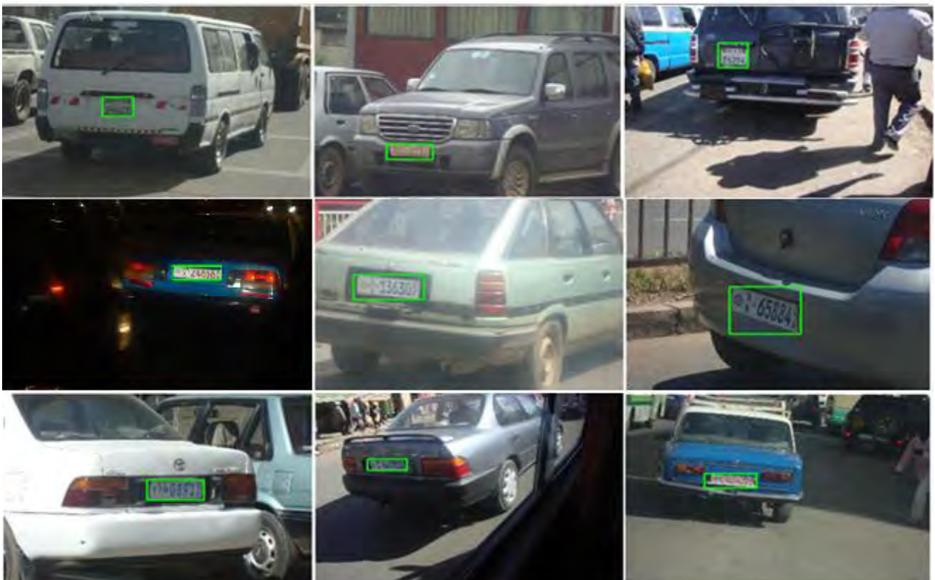
Figure 4.1: Sample successful plate detection instances
