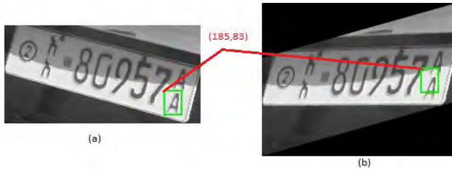
Figure 3.15: Presents the outcome of the spatial transformation (i.e., Shear transform) on (b) performed on (a).
