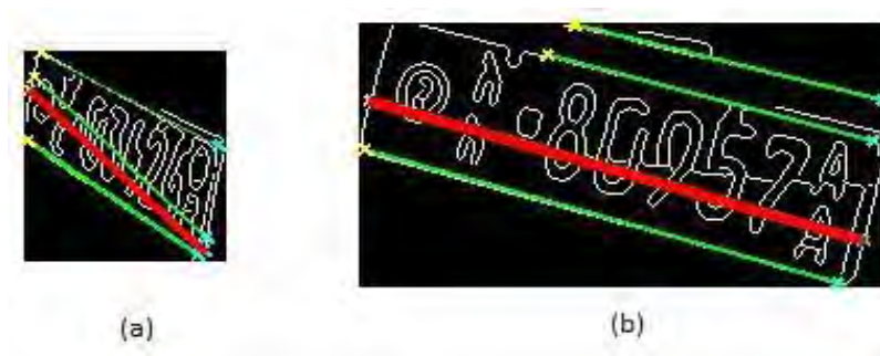
Figure 3.14 Response of linear Hough transform, labeling the longest line red.
