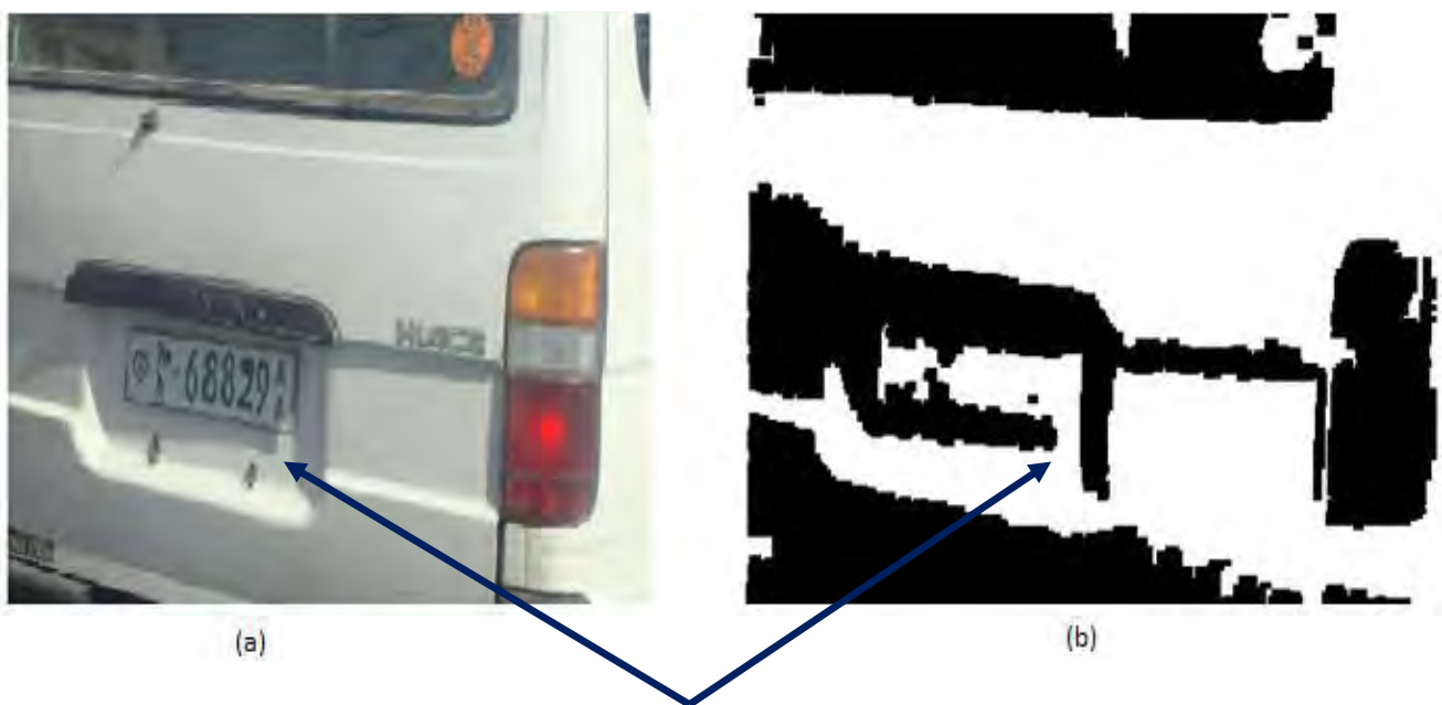
Figure 4.2: An instance where the PD module fails to detect plate region, because of shadow effects
