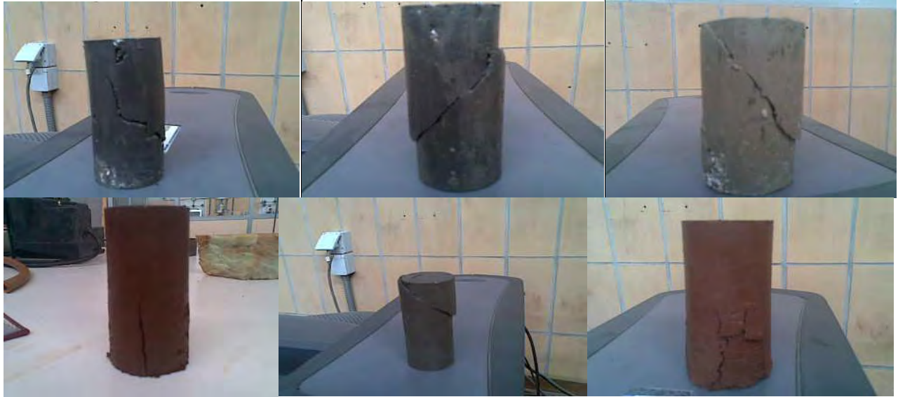
Fig 4.9 - Typical appearance of failed specimens after unconfined compressive strength testing
