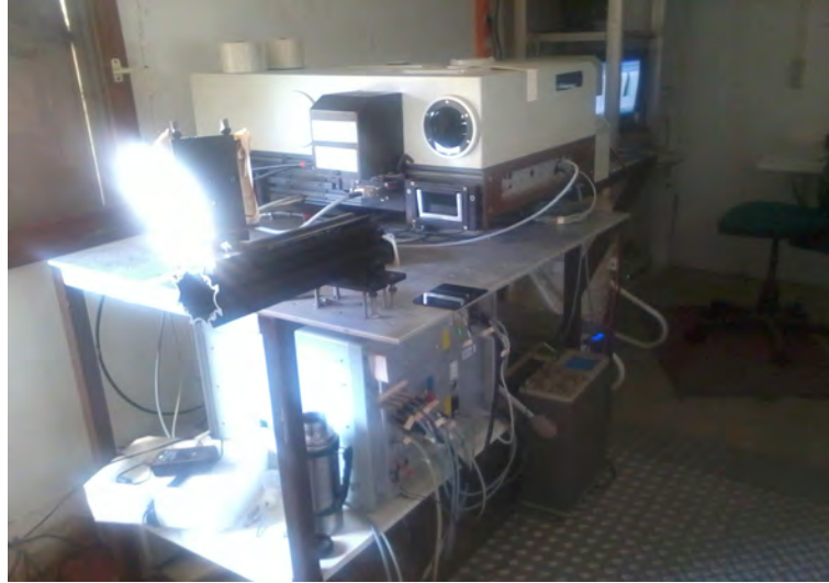
Figure 3.1: The FTIR spectrometer at measurement site in Addis Ababa.
