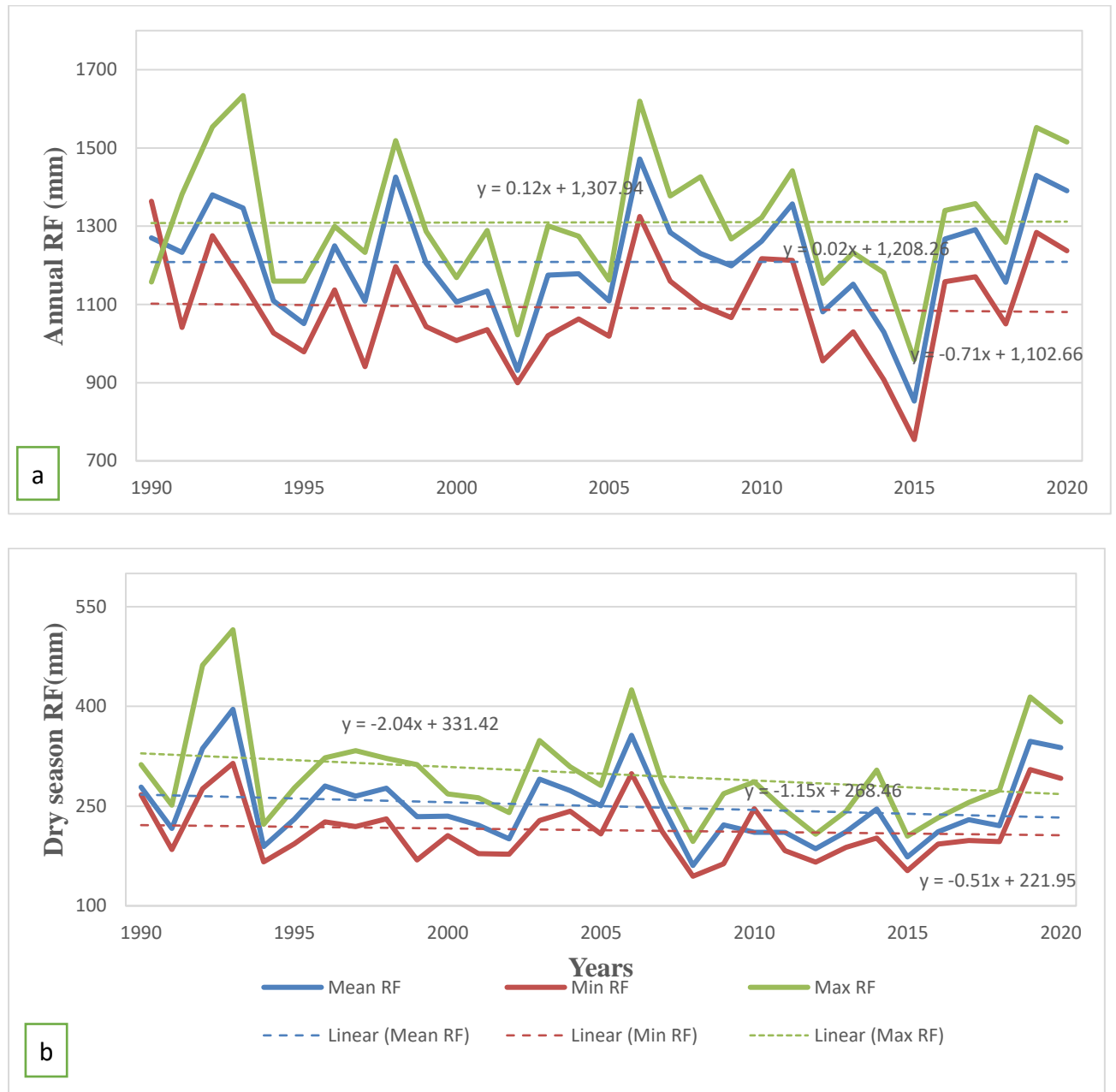
Figure 16: Trend line of mean, minimum and maximum Annual (a) and dry season rainfall (b) from 1990 to 2020
