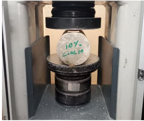
Figure 4.4 Universal Testing Machine setup for Splitting Tensile Strength Test.
