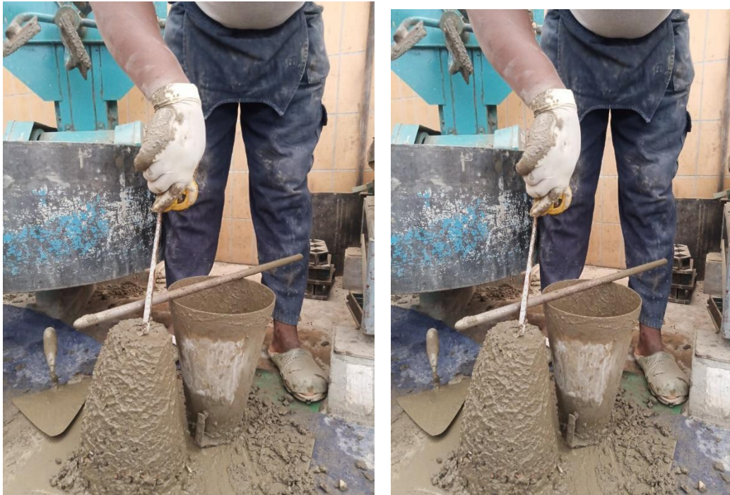
Photo 5. Slump test without ceramic (left) and with ceramic (right)
