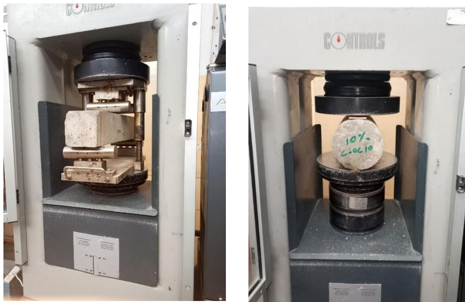
Photo 10. Flexural Strength test (left) and Splitting Tensile Strength test (right)
