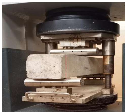
Figure 4.5 Universal Testing Machine setup for Flexural Strength Test.
