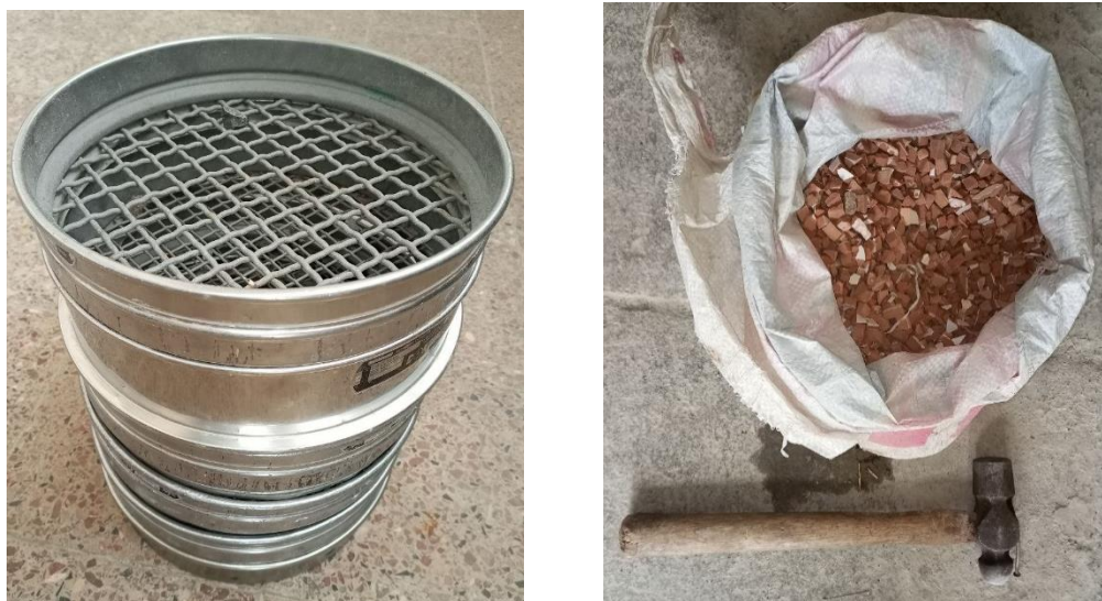
Photo 2. Sieves (left) and Ball-peen Hammer (right) used to crush waste ceramic.
