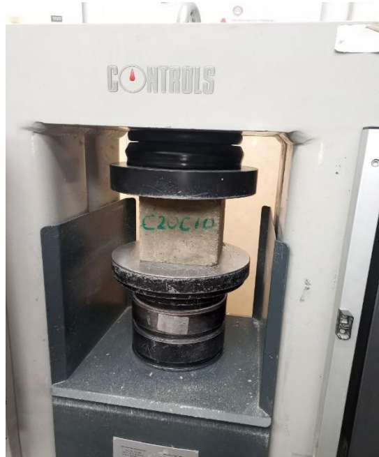
Figure 4.3 Universal Testing Machine setup for Compression Strength Test.
