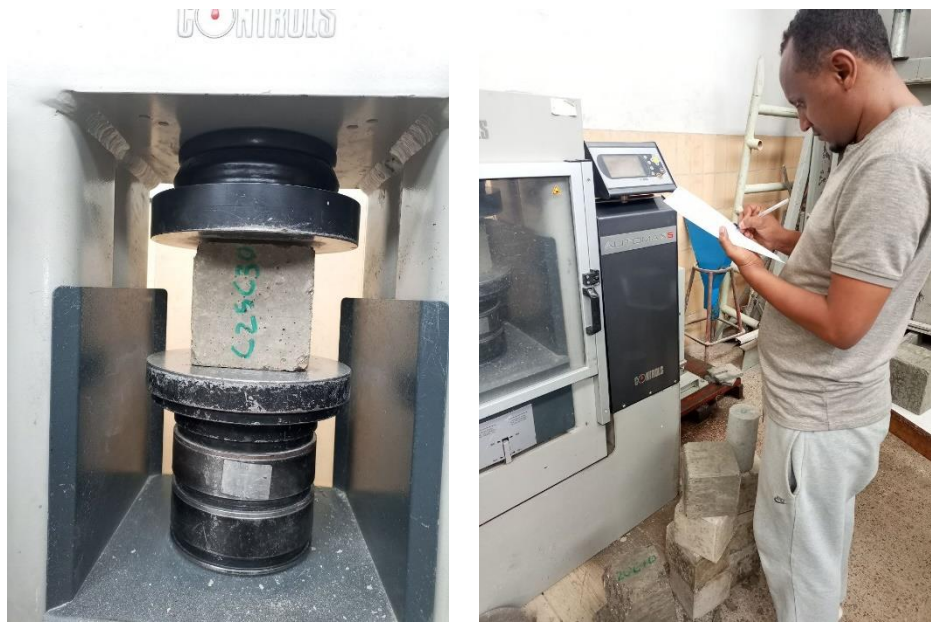
Photo 9. Compressive Strength test.
