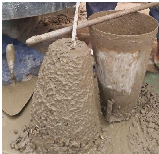
Figure 4.2 Workability test of concrete.
