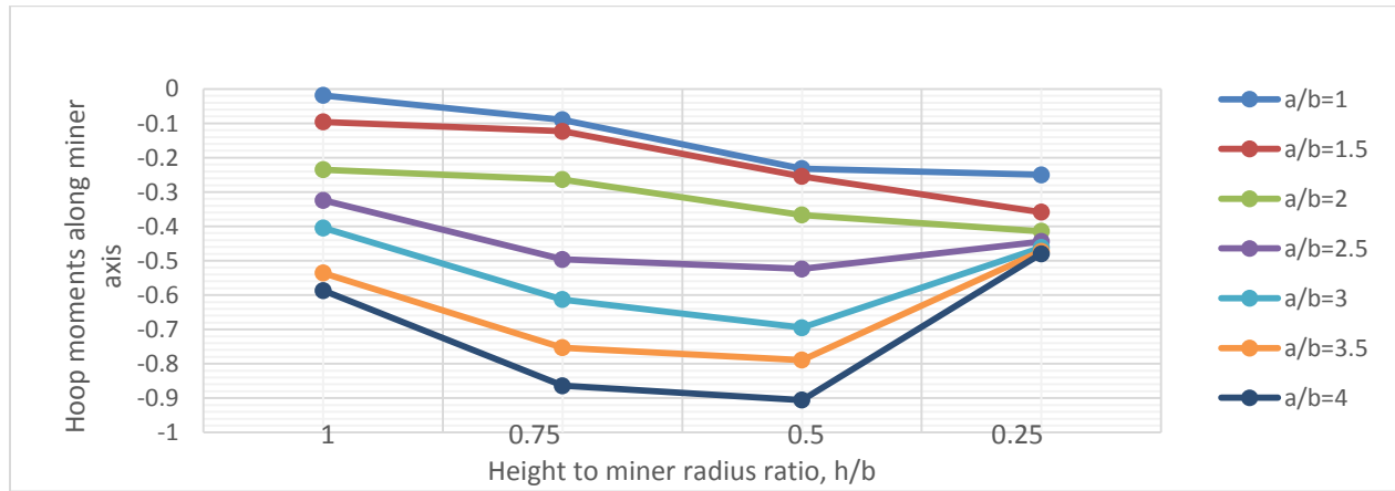
Figure 3.25 influence of aspect ratio for hoop moments along miner axis
