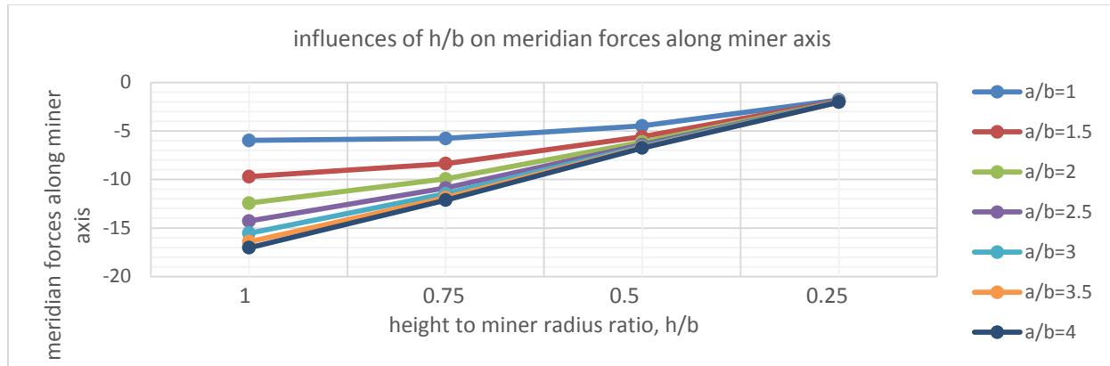
Figure 3.12 influence of height to miner radius ratio for meridian forces along miner axis
